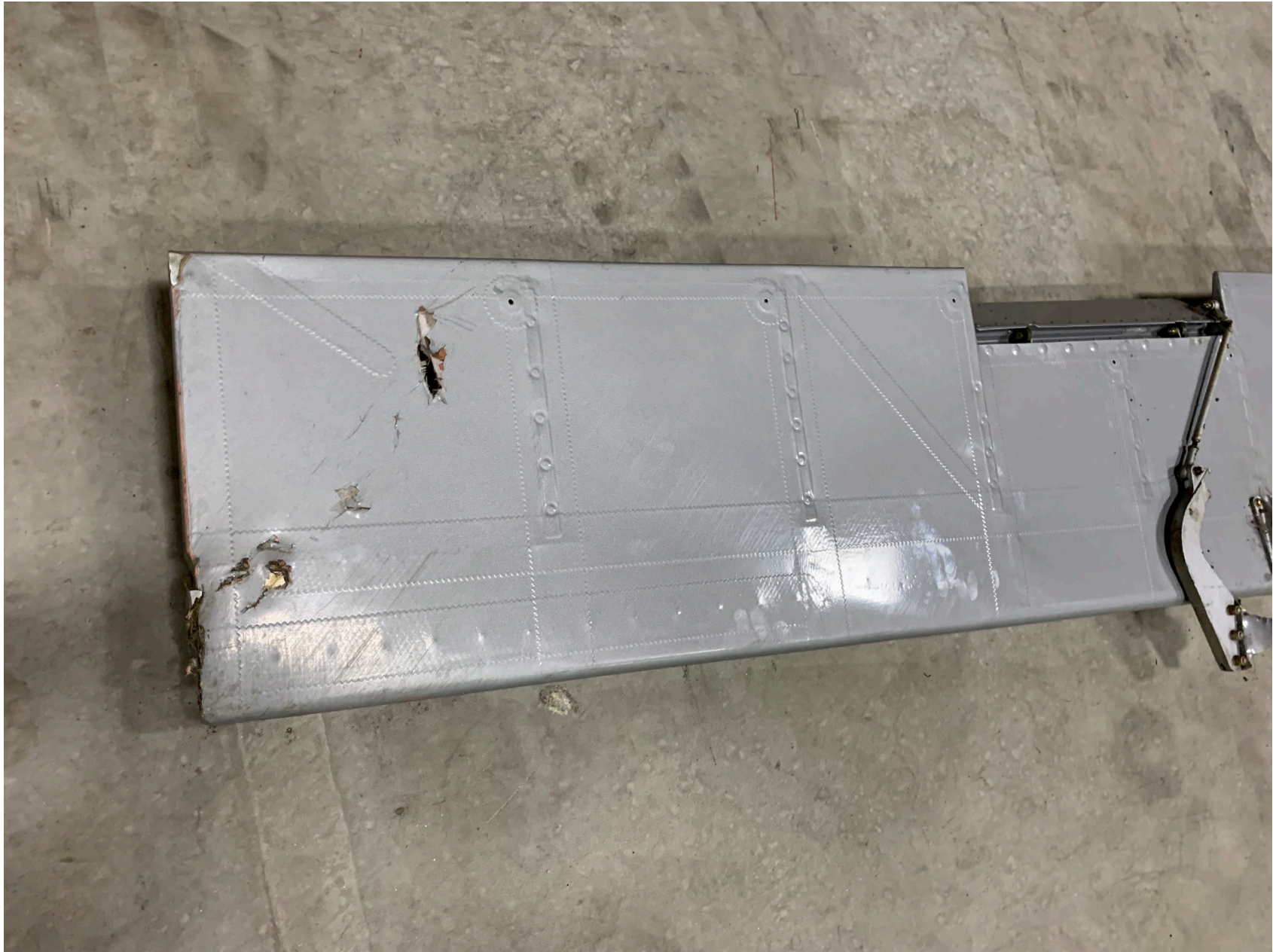
Photo 3 -Substantially damaged left aileron (Photo Provided by FAA)
