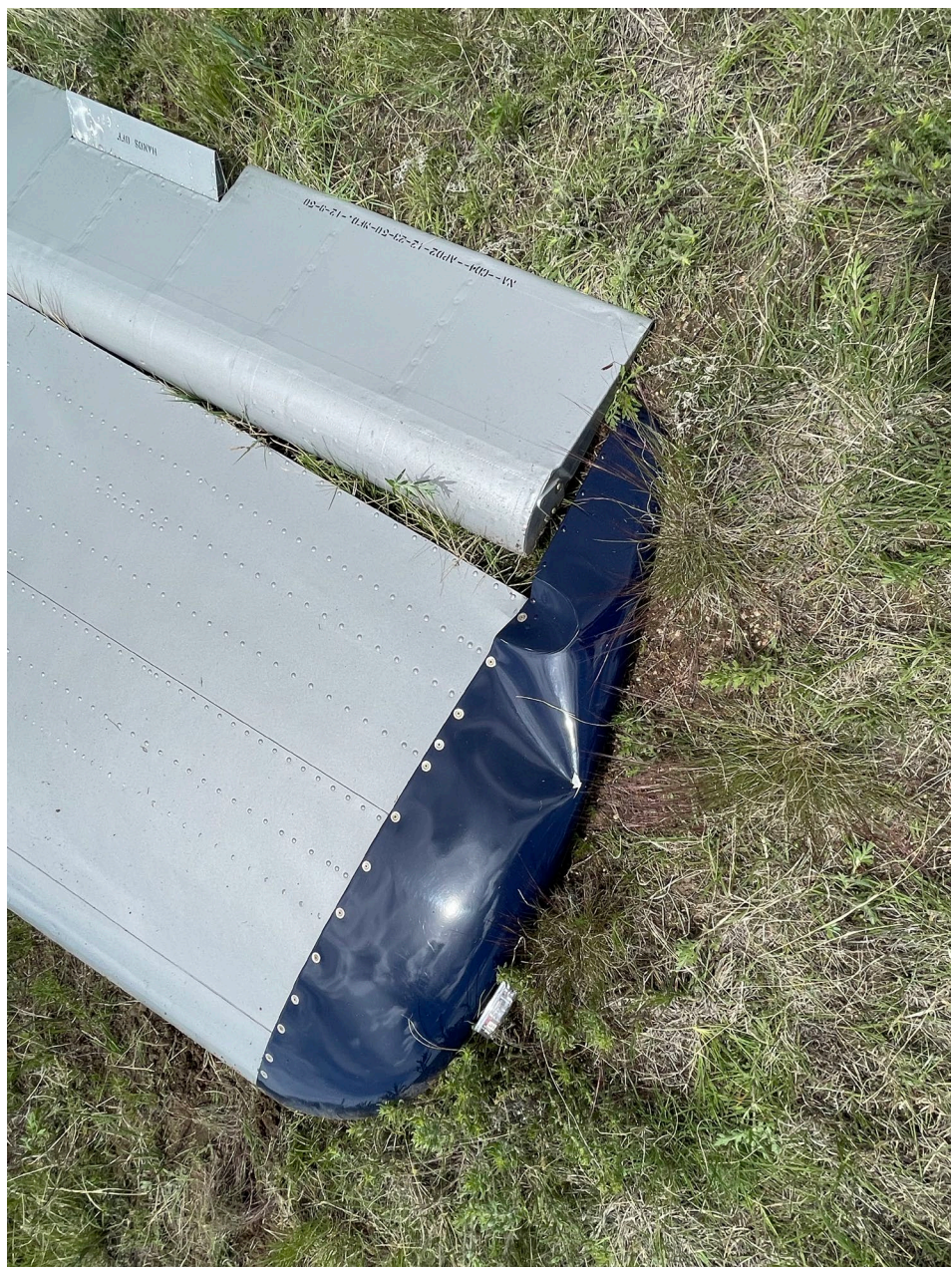
Photo 2 – Substantially damaged left wing and aileron (Photo Provided by FAA)
