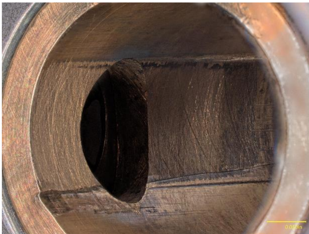
Figure 9. Witness marks on ID of cam bushing
