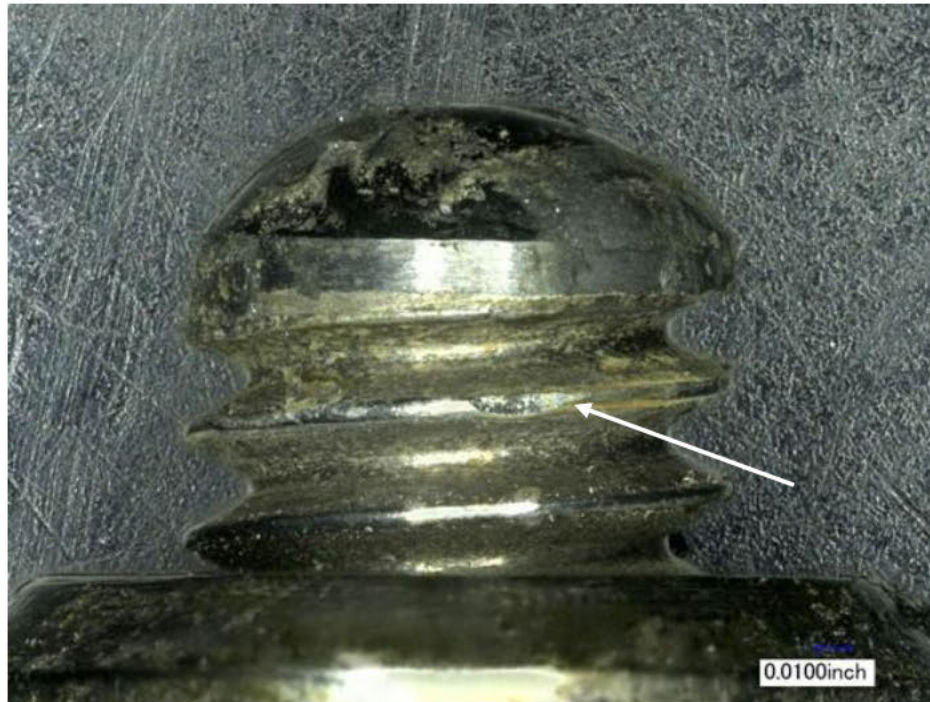
Figure 11. Damage on cam follower thread
