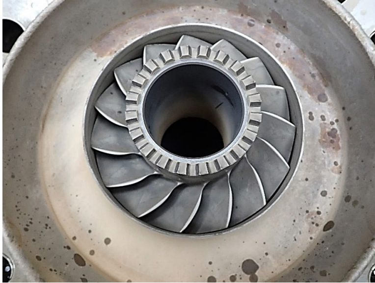
Photo 28. Forward End (Inducer) of the Stage 2 Impeller (Installed)
