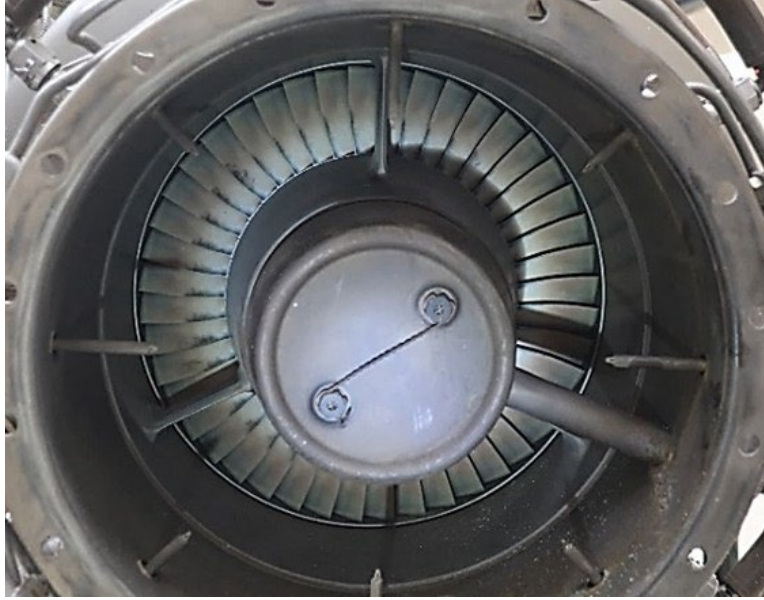
Photo 4. Power Turbine Rotor/Blades - Looking Through Exhaust Duct
