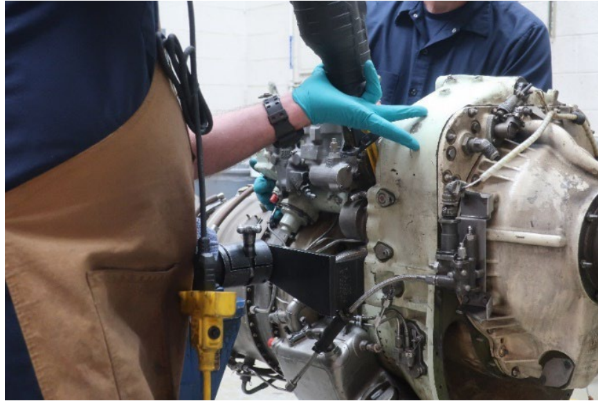
Photo 13. Removal of the Fuel Control Unit
