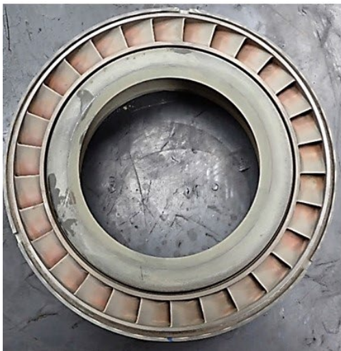
Photo 23. Stage 1 Nozzle (L) with Trailing Edge Cracks (R)
