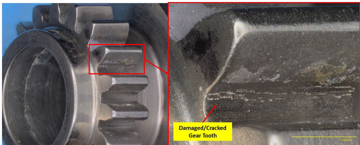
Photo 44. Cam Shaft Gear - Damaged Tooth
