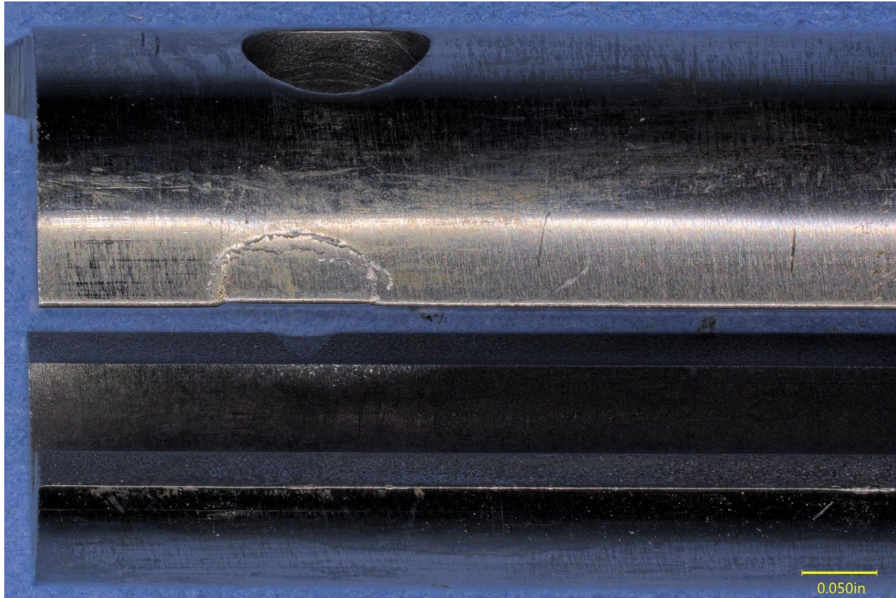
Figure 25. View of the damaged areas of the slot corners after cleaning and grease removal, viewed from slot 2.
