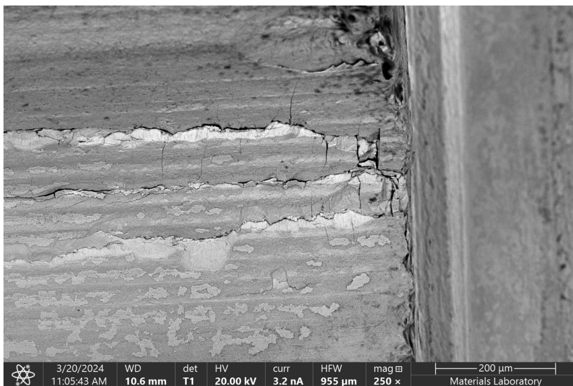
Figure 74. BE micrograph of the fillet radius of the gear tooth, showing longitudinal cracking.
