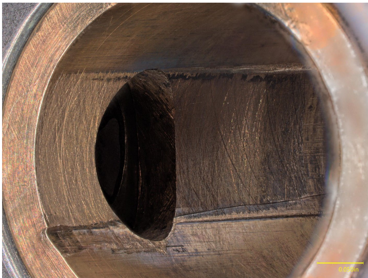
Figure 56. Angled view of the bushing interior that mated with slot 1 of the shaft, after cleaning.
