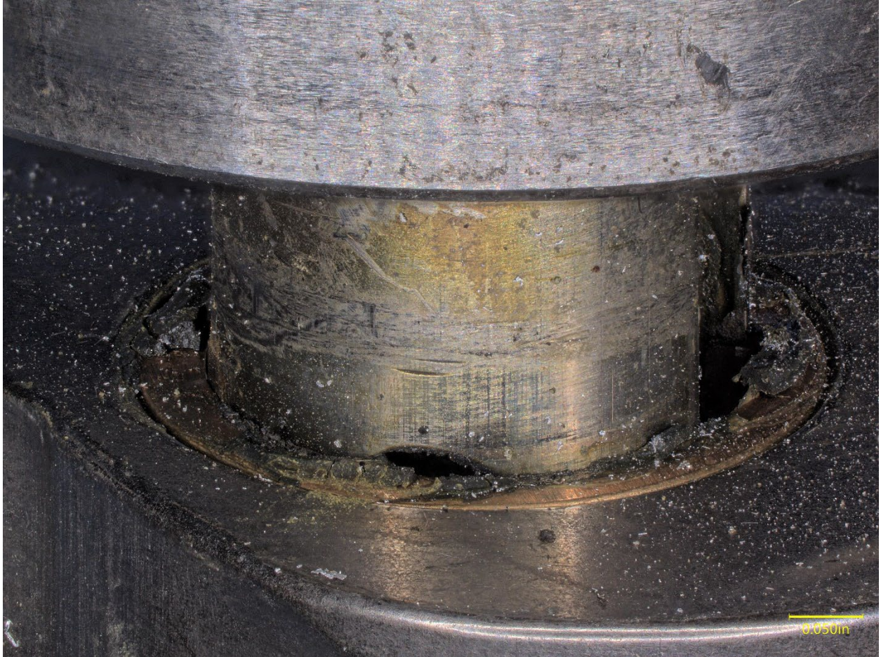
Figure 8. Angled view of the shaft and camgear face from the pinion side of the shaft, showing the pinhole.
