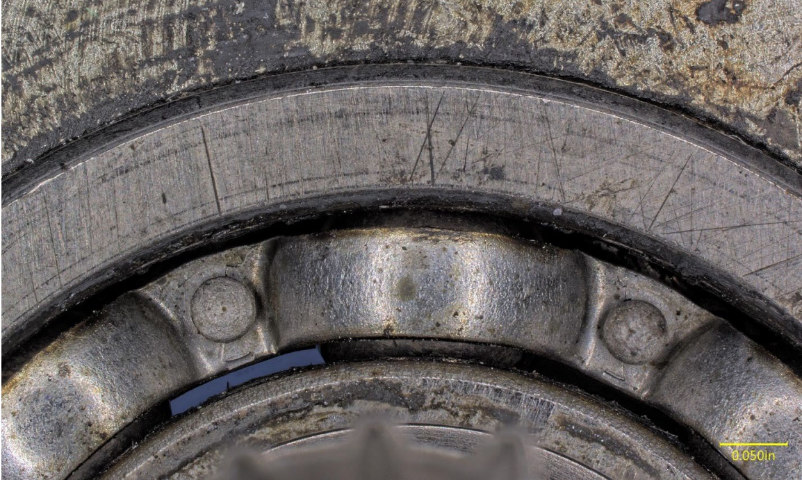
Figure 64. Closer view of the cage and roller balls inside the bearing in Figure 56.
