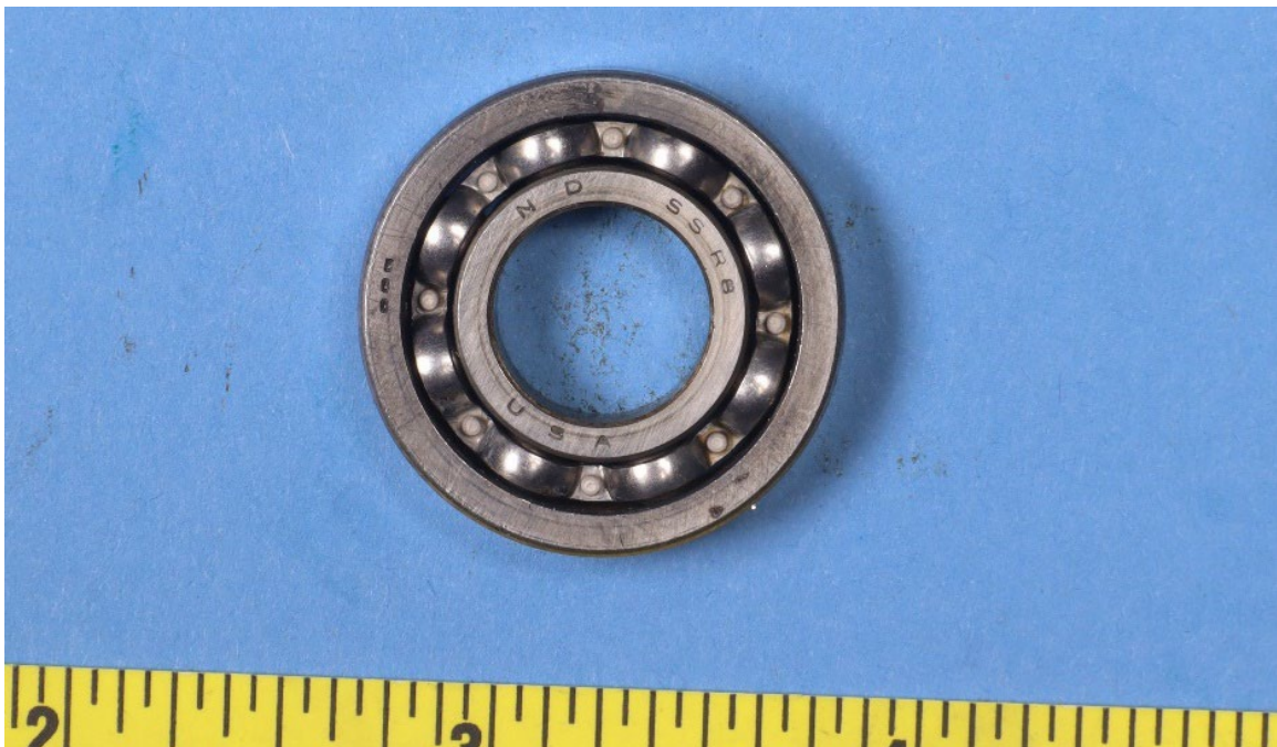
Figure 63. View of the bearing after removal from the camshaft assembly.
