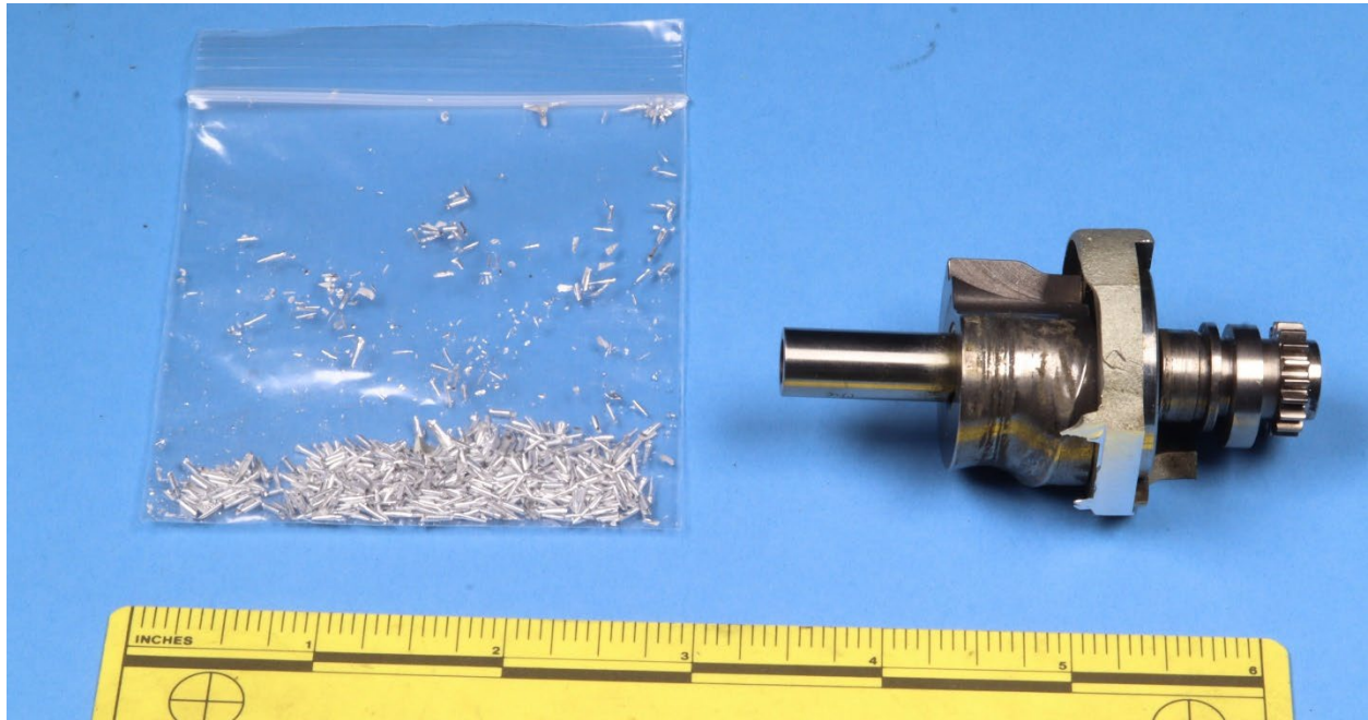
Figure 1. The camgear/camshaft assembly and a bag of metallic debris, as received.
