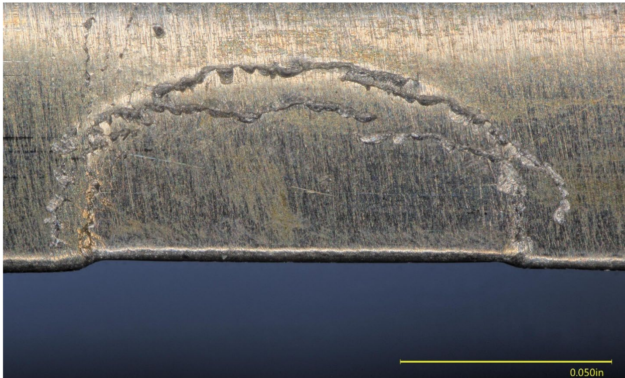
Figure 41. View of the damaged area in the corner of slot 2, after full cleaning.
