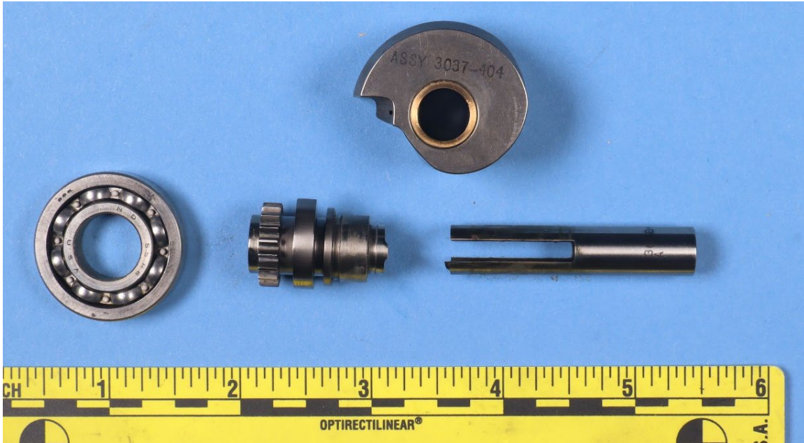
Figure 17. View of the camshaft, camgear, and bearing after sectioning and disassembly.
