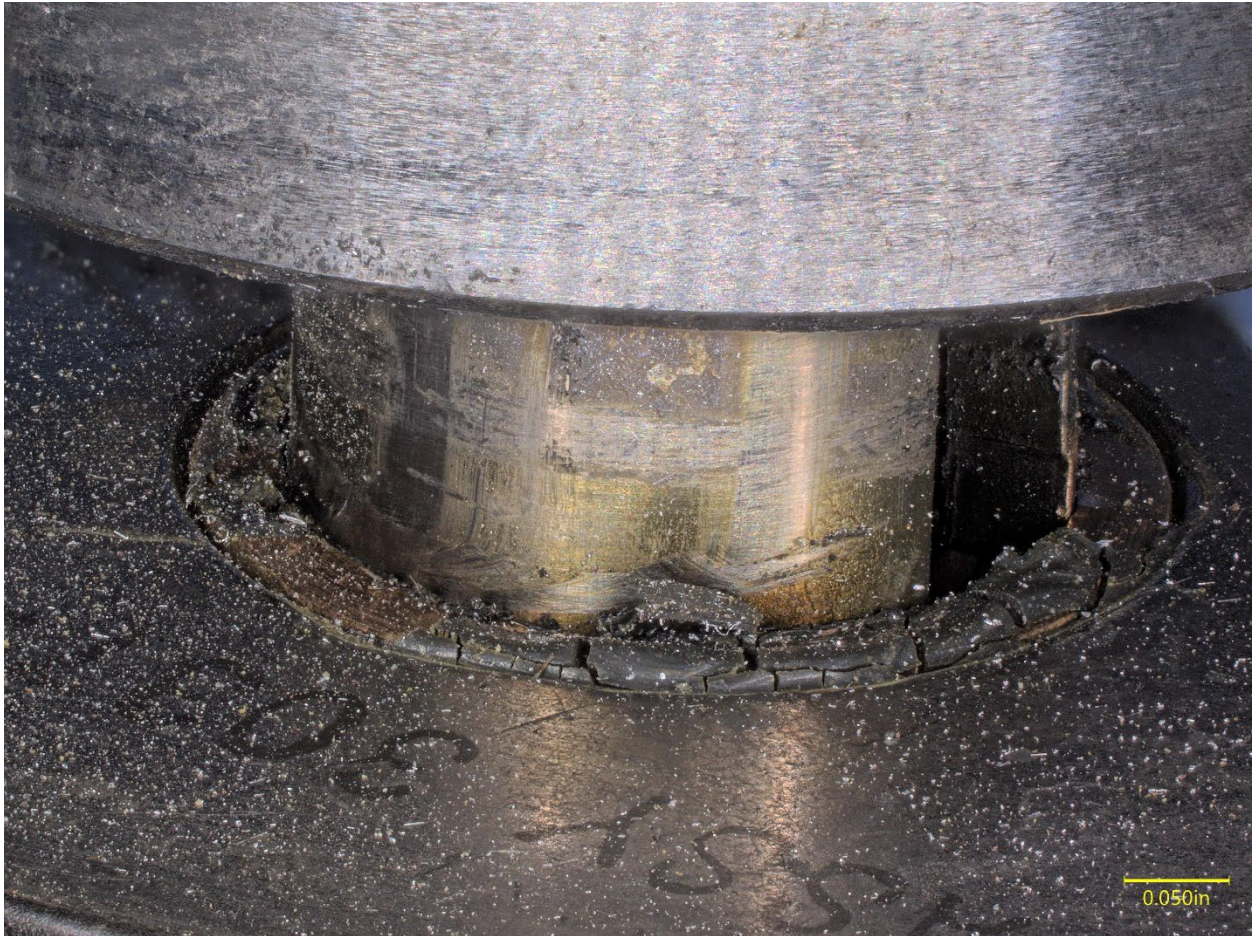
Figure 6. Angled view of the shaft and camgear face from the pinion side of the shaft, showing slot 2.
