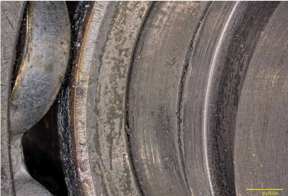
Figure 65. Angled view of the inner race outer surface with the cage, showing darker deposits between the surface.
