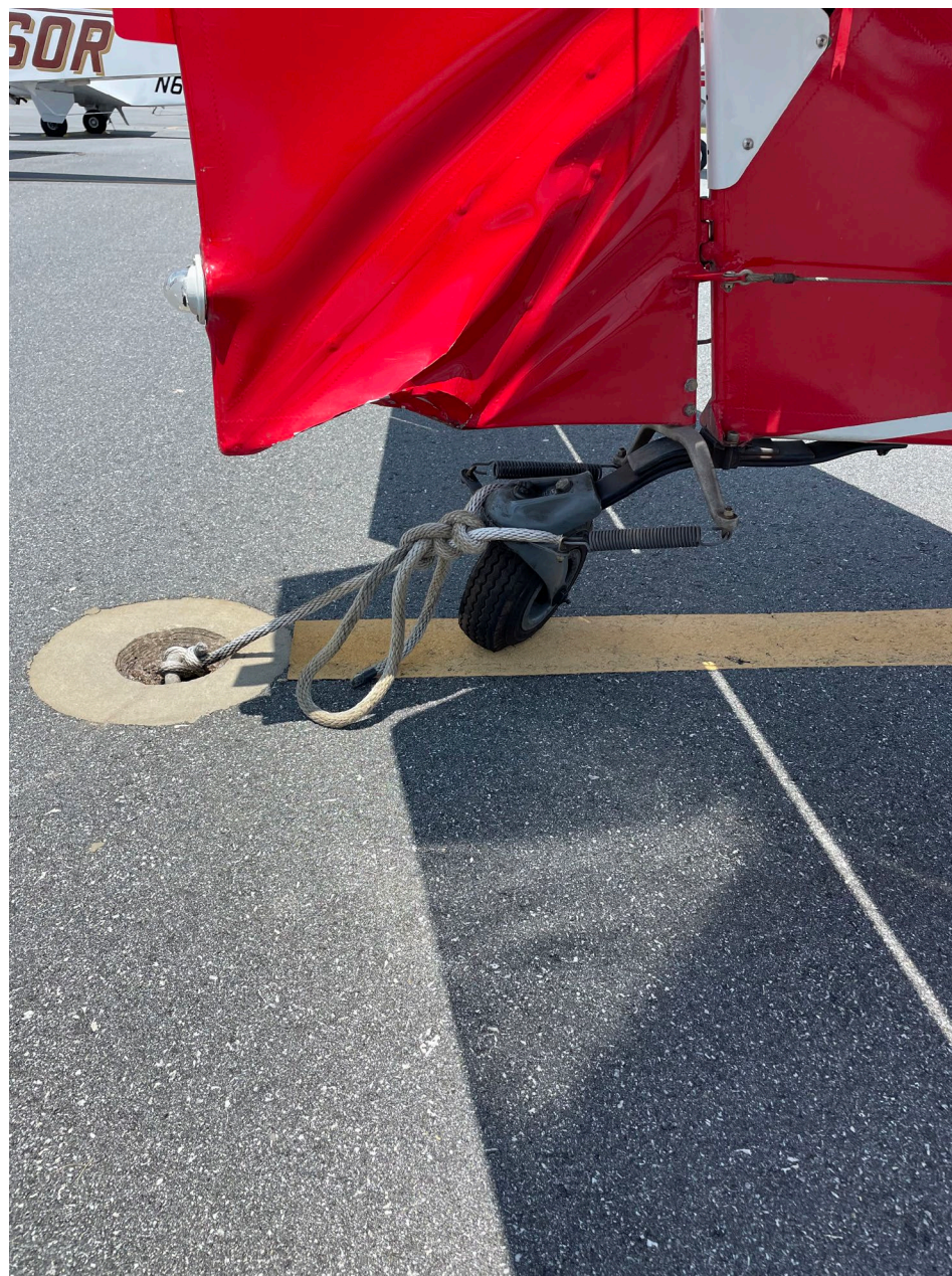
Photo 2 - Damaged Rudder of Accident Airplane (FAA)
