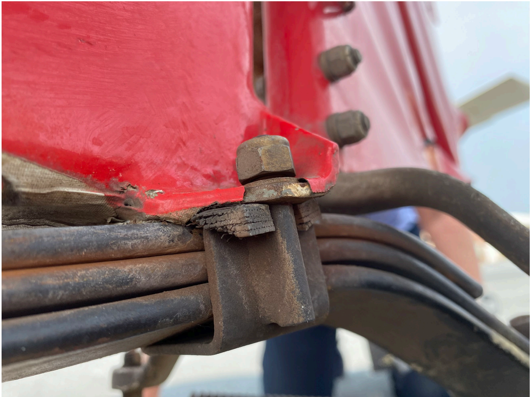
Photo 3 – Loose Tailwheel Spring Attachment Hardware (FAA)
