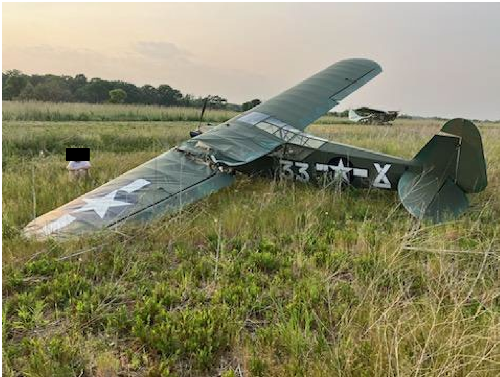
Photo 1 – Airplane with damaged left wing (Photo provided by FAA)
