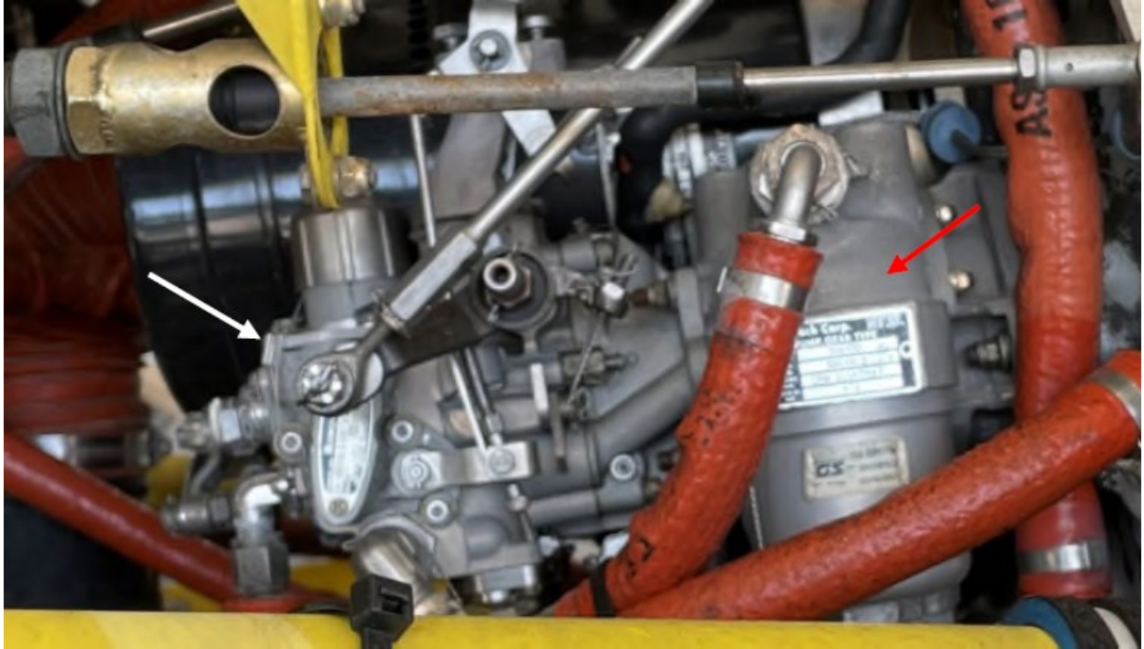
Figure 32 - Fuel Pump and FCU
