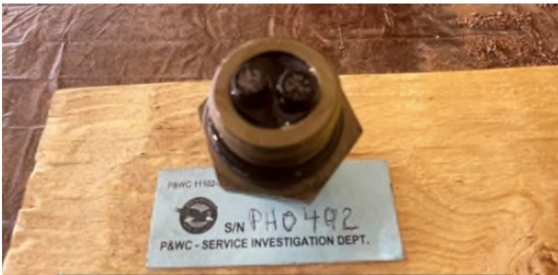
Figure 20 - Magnetic Chip Detector
