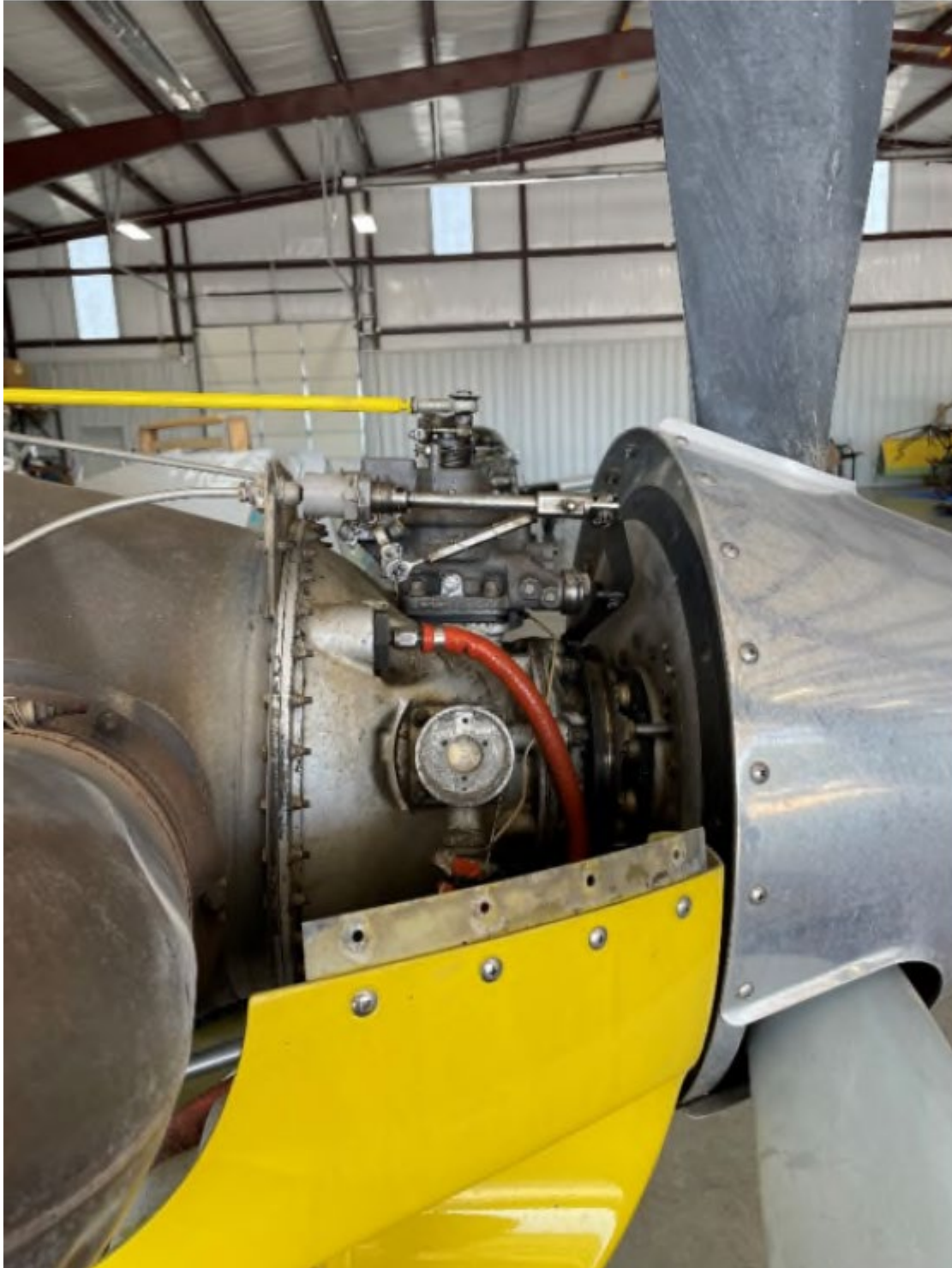
Figure 4 - Reduction Gear Box
