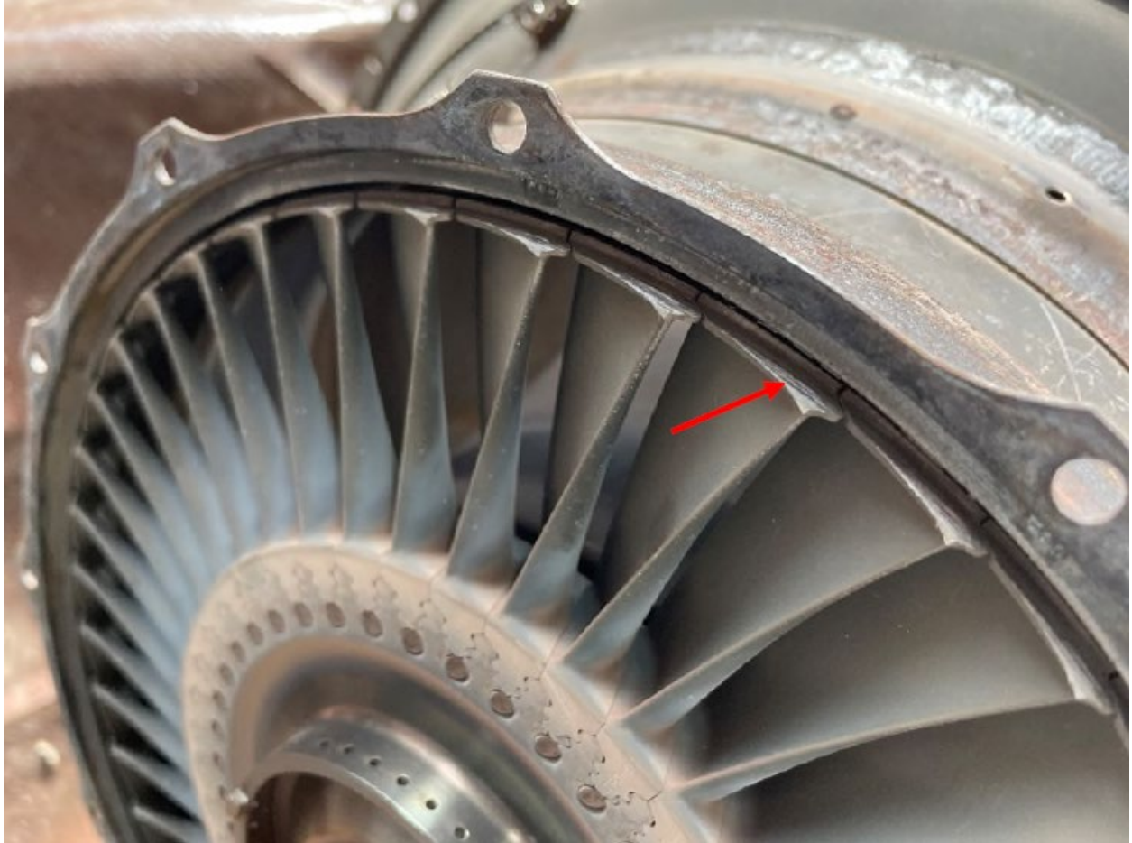
Figure 27 - PT vane ring outer shroud lip
