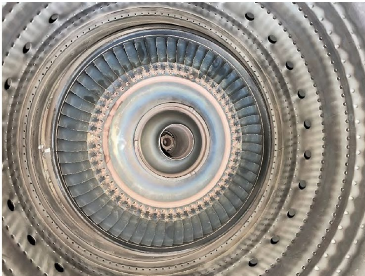
Figure 22 - CT disc and blades
