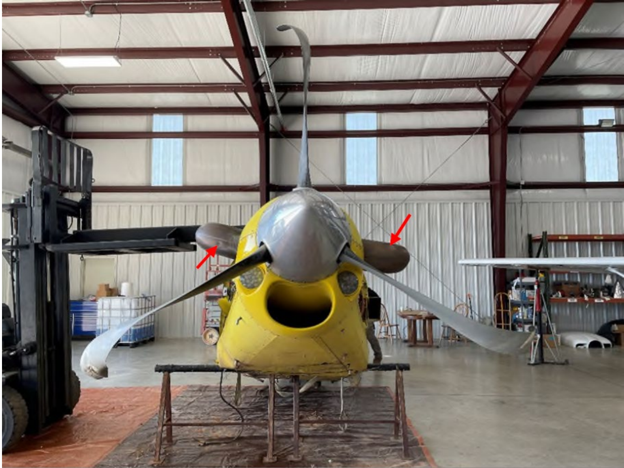
Figure 2 - Propeller and exhaust stacks
