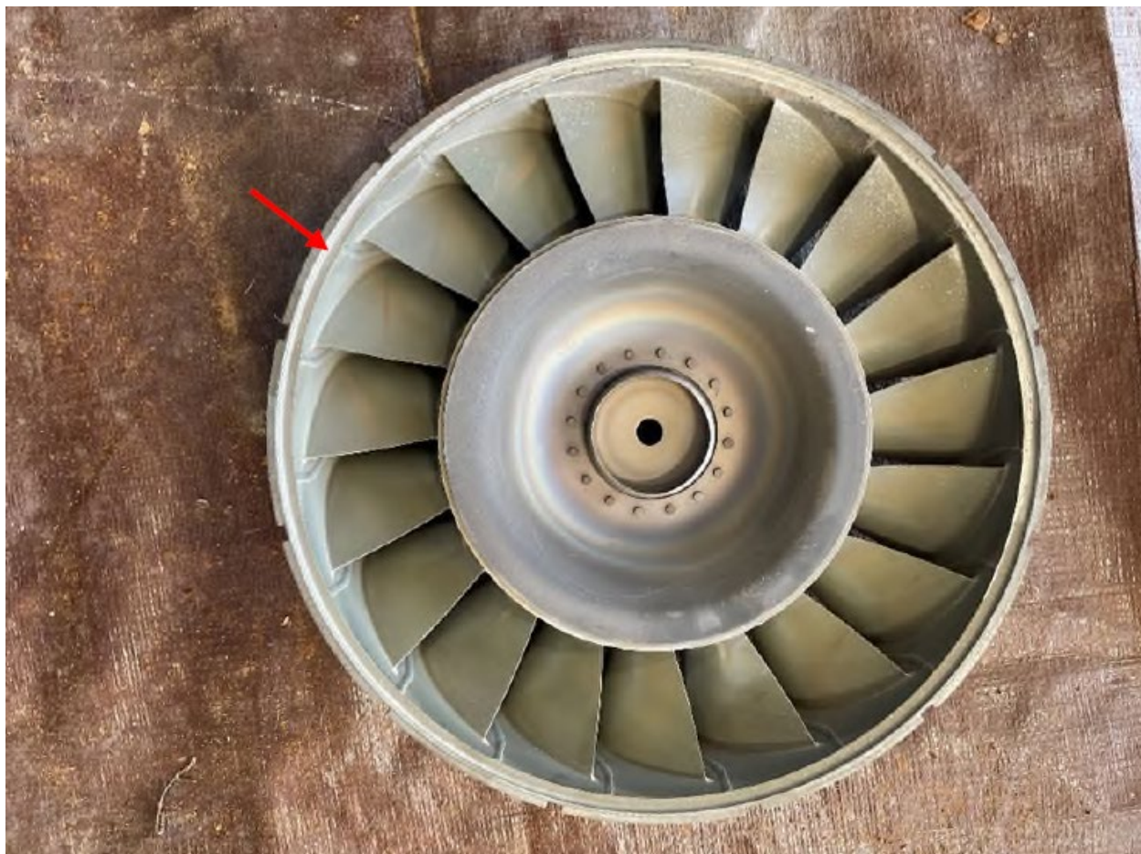
Figure 25 - PT Vane Ring Downstream
