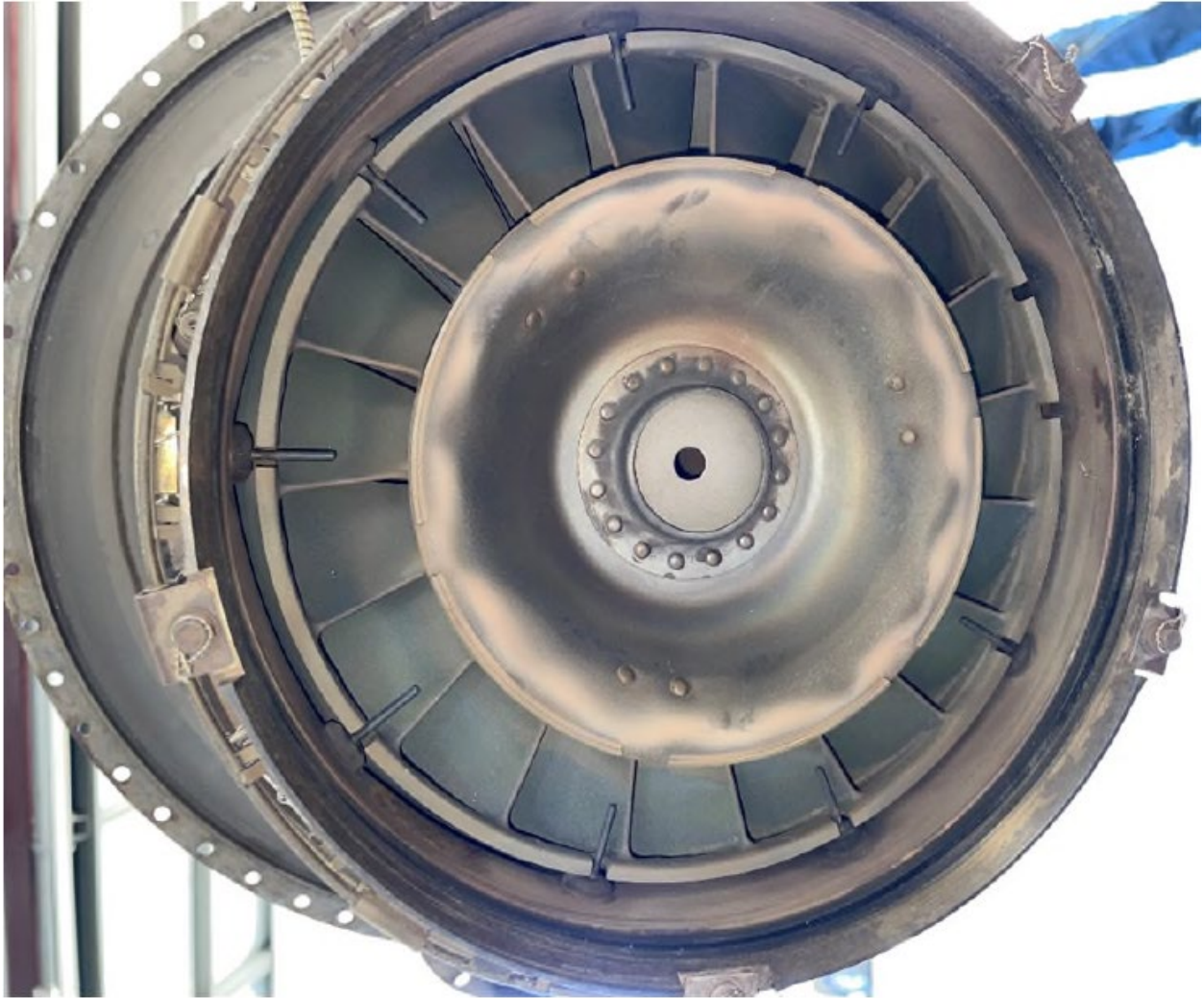
Figure 24 - PT Vane Ring, ITT Probes and Busbar
