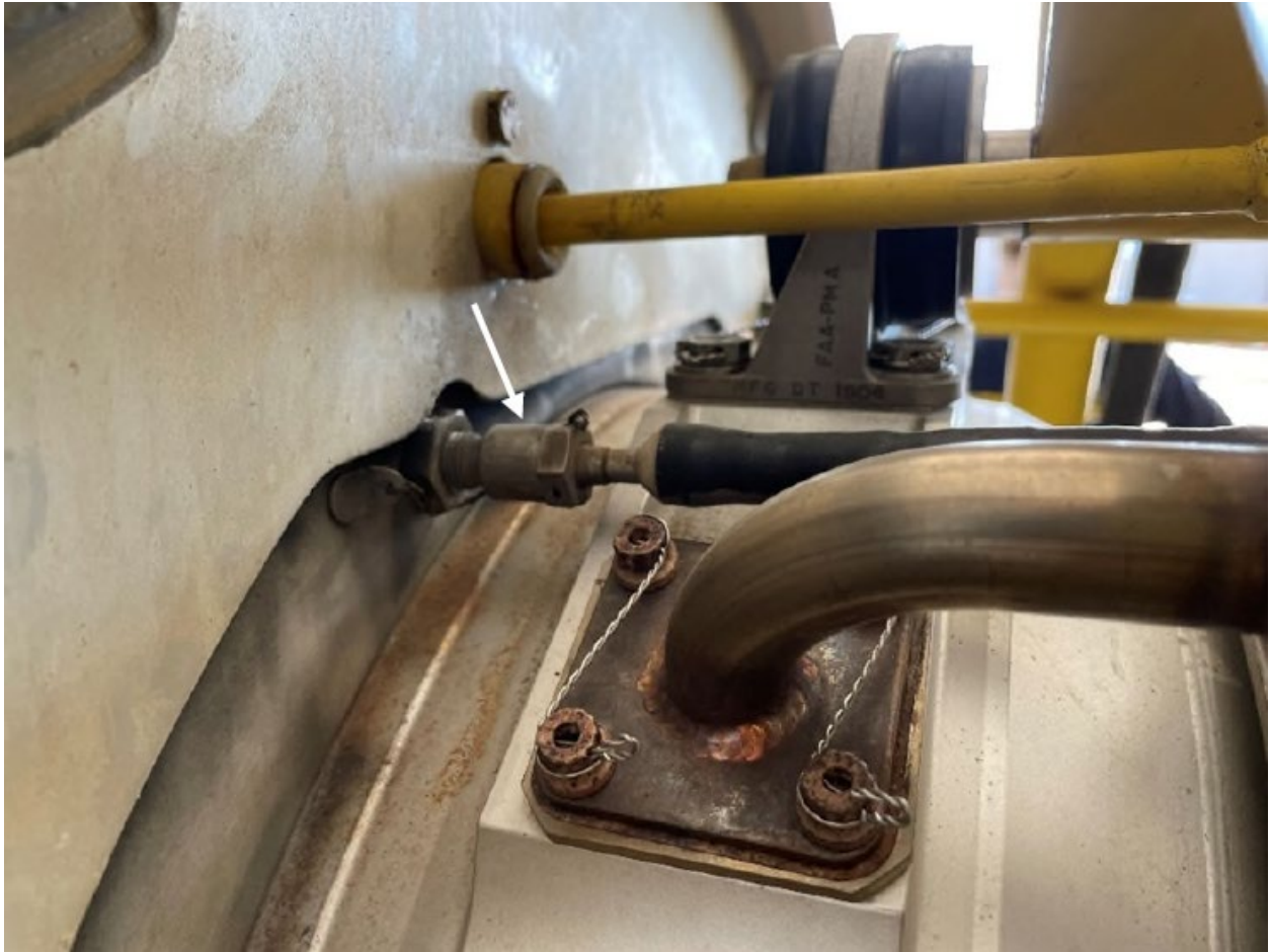
Figure 18 - Py Fitting at Front Firewall
