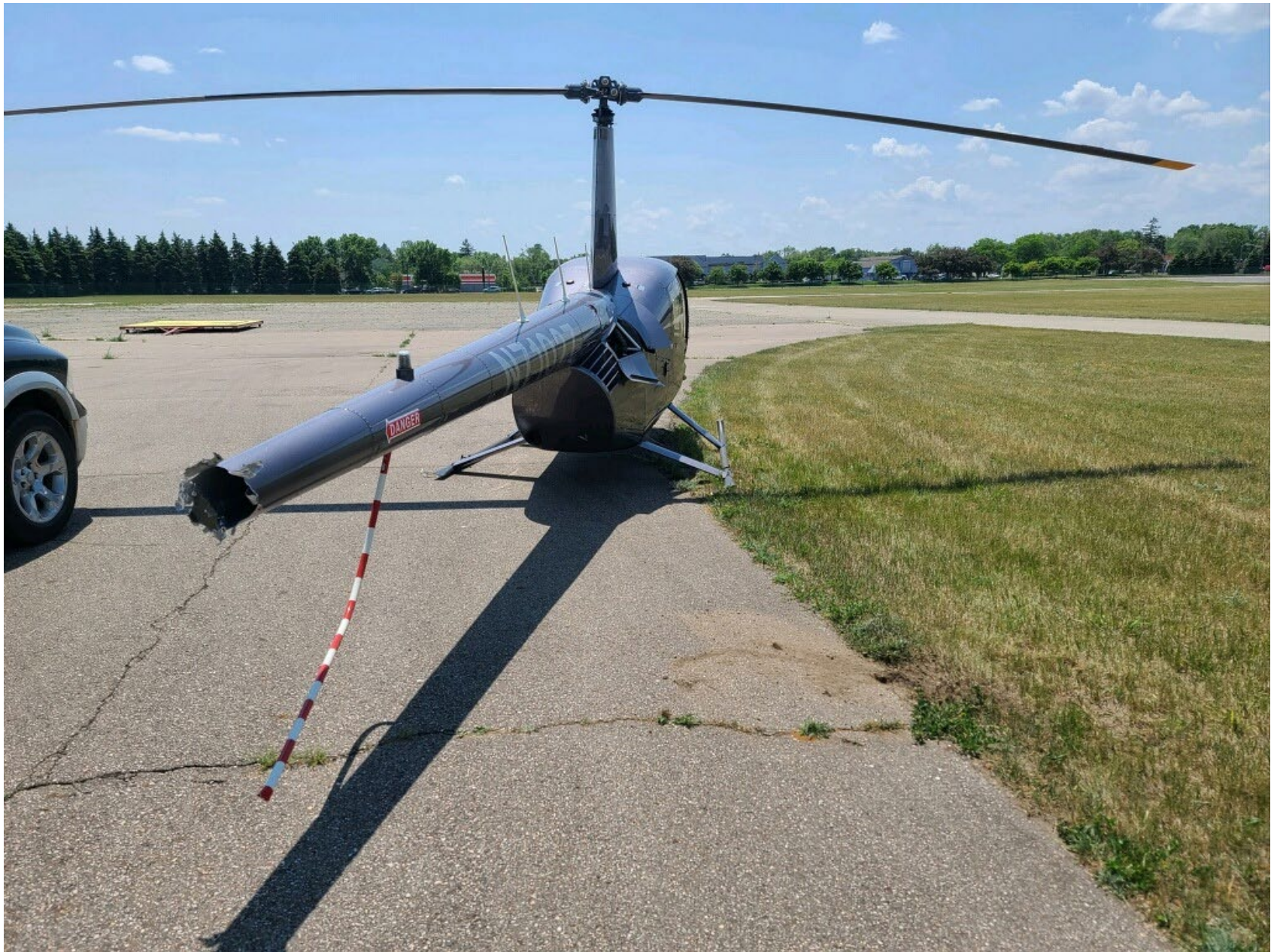
Photo 2 – View of substantially damaged tailboom (Photo Provided by Flight Instructor)
