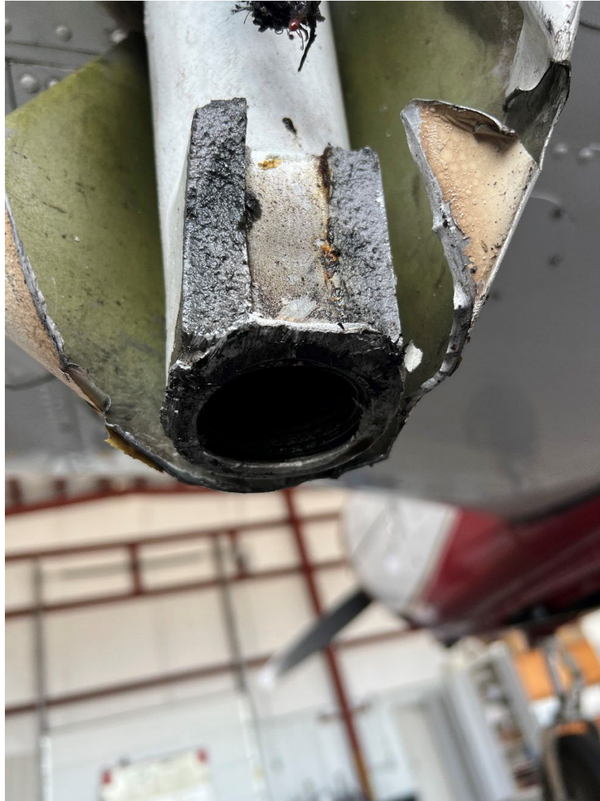
Photograph 1 - Fractured left main landing gear strut housing clevis (Courtesy of the Federal Aviation Administration)
