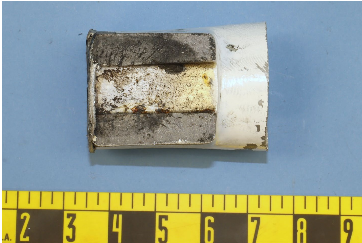
Figure 2. View of the fracture surface from the sectioned side of the upper cylinder.
