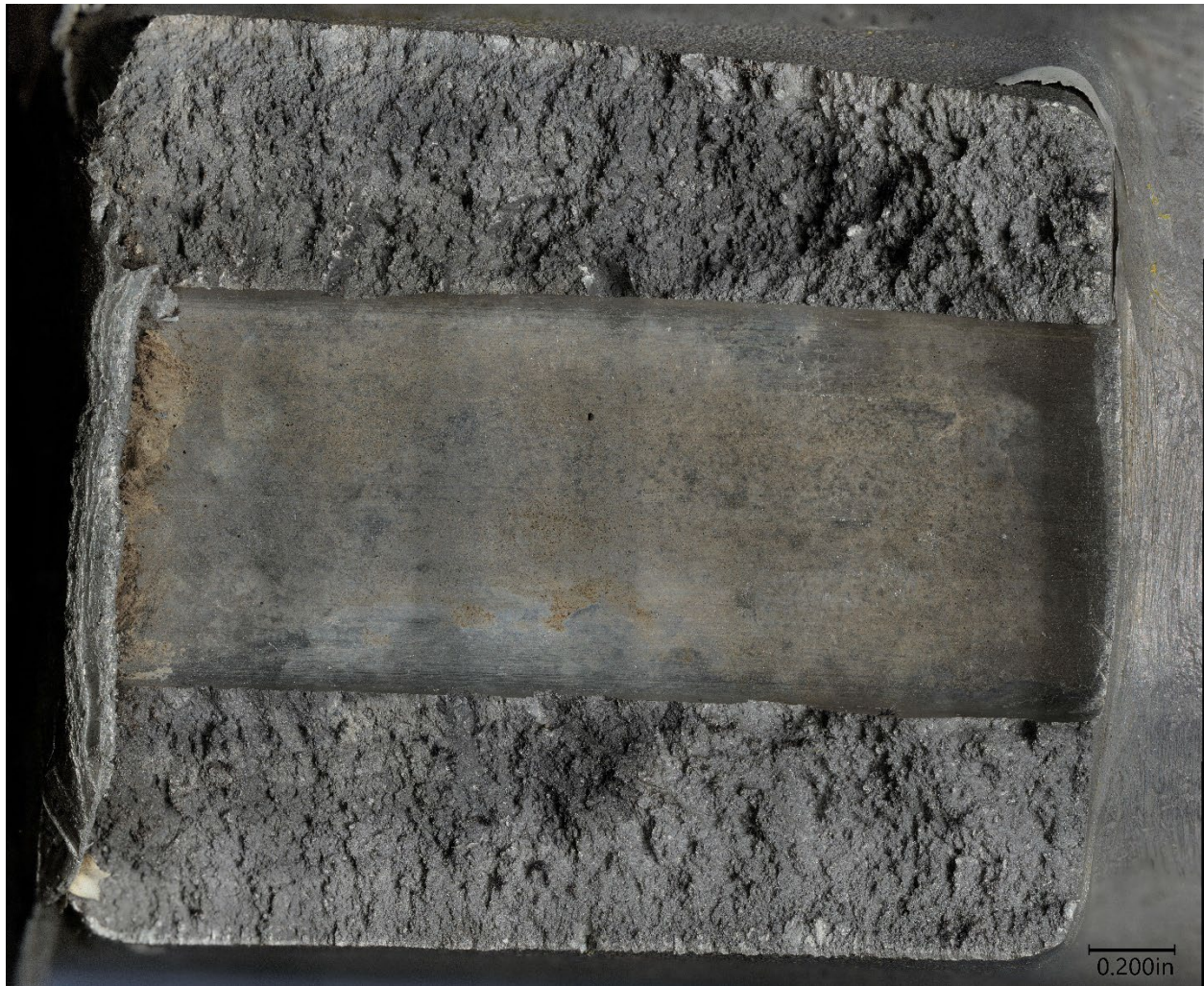
Figure 4. Montage of the connection fracture surface in Figure 3, showing the difference in color between the progressive and instantaneous regions.
