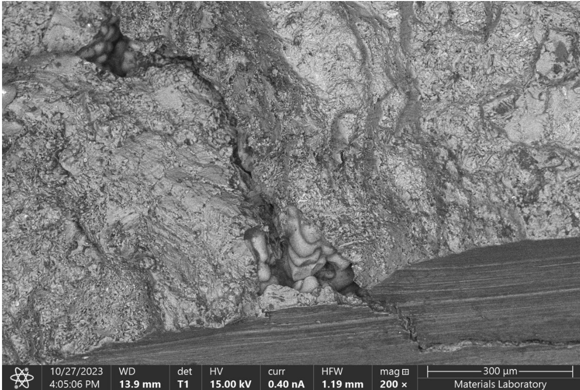
Figure 15. BE micrograph of a secondary crack along a void at the fracture edge.
