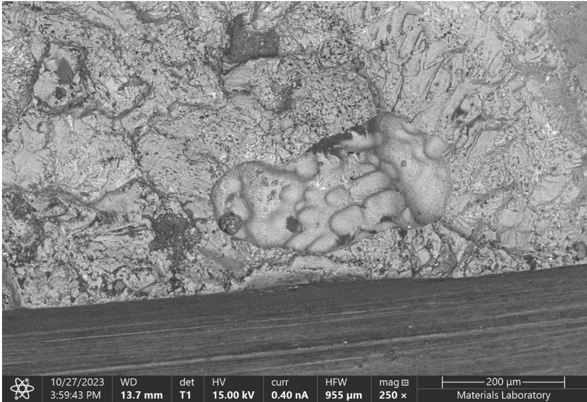
Figure 13. Backscattered electron (BE) micrograph of a void near the fracture surface edge.
