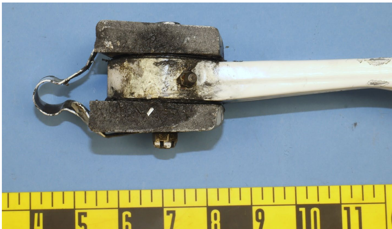
Figure 3. Mating cylinder clevis fracture surfaces from Figure 2, still affixed to the strut remnant.
