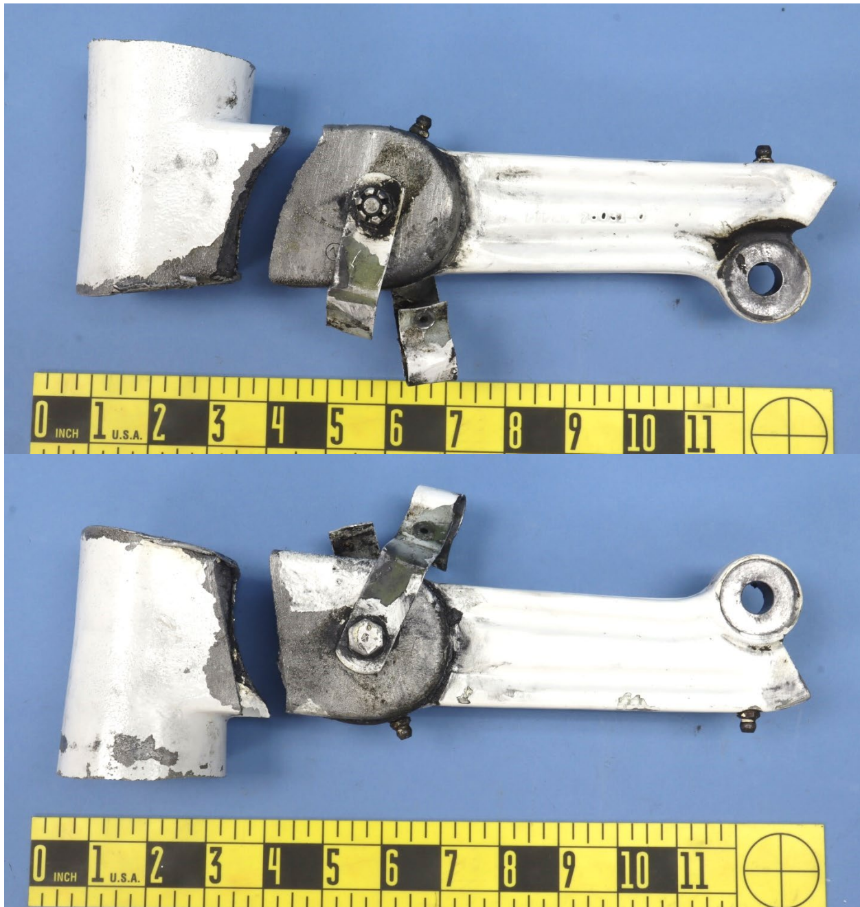
Figure 1. View of the opposite sides of the fractured strut assembly clevis remnants attached to the torque link arm, and the sectioned cylinder remnant, as received.
