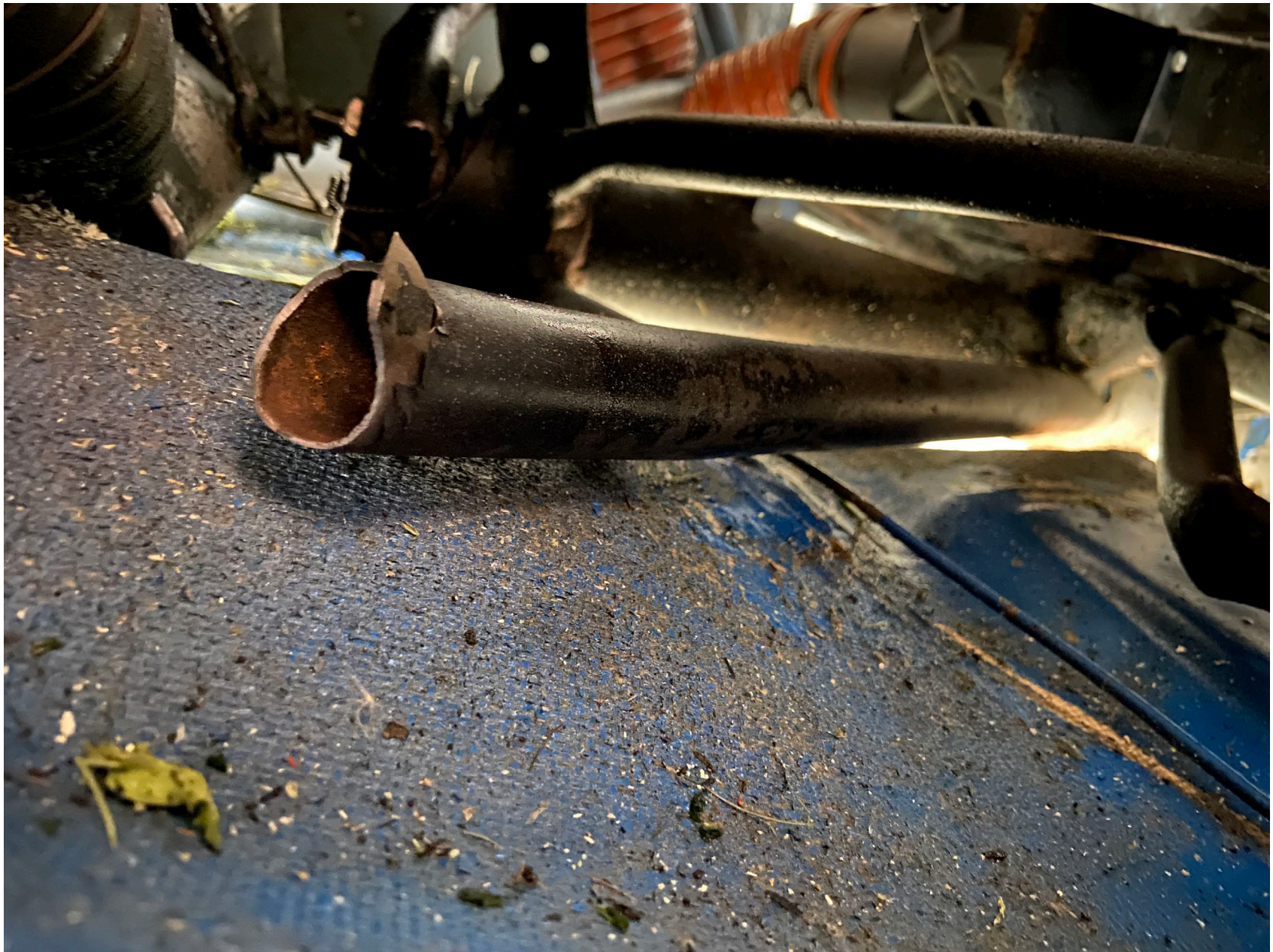
Photo 2 – Broken engine mount (Photo from FAA)
