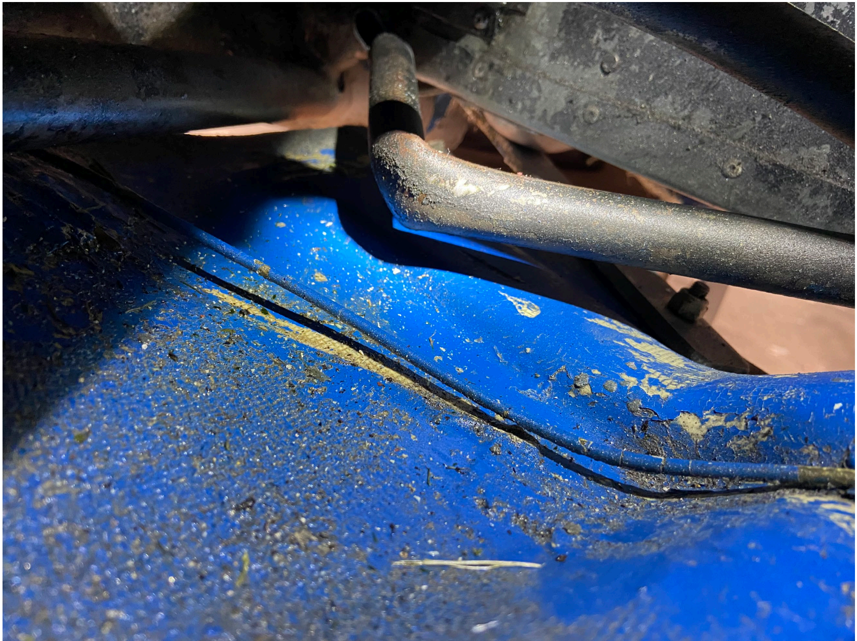
Photo 1 – Bent engine mount (Photo from FAA)
