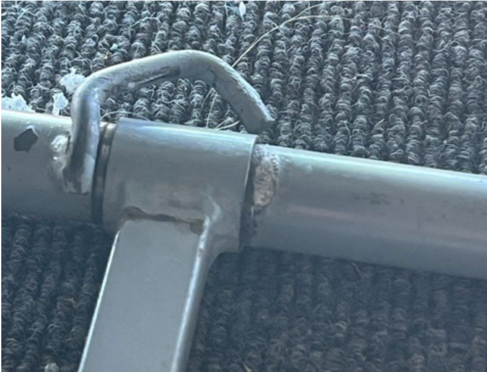
Photograph 8 - Failed weld (Courtesy of FAA)
