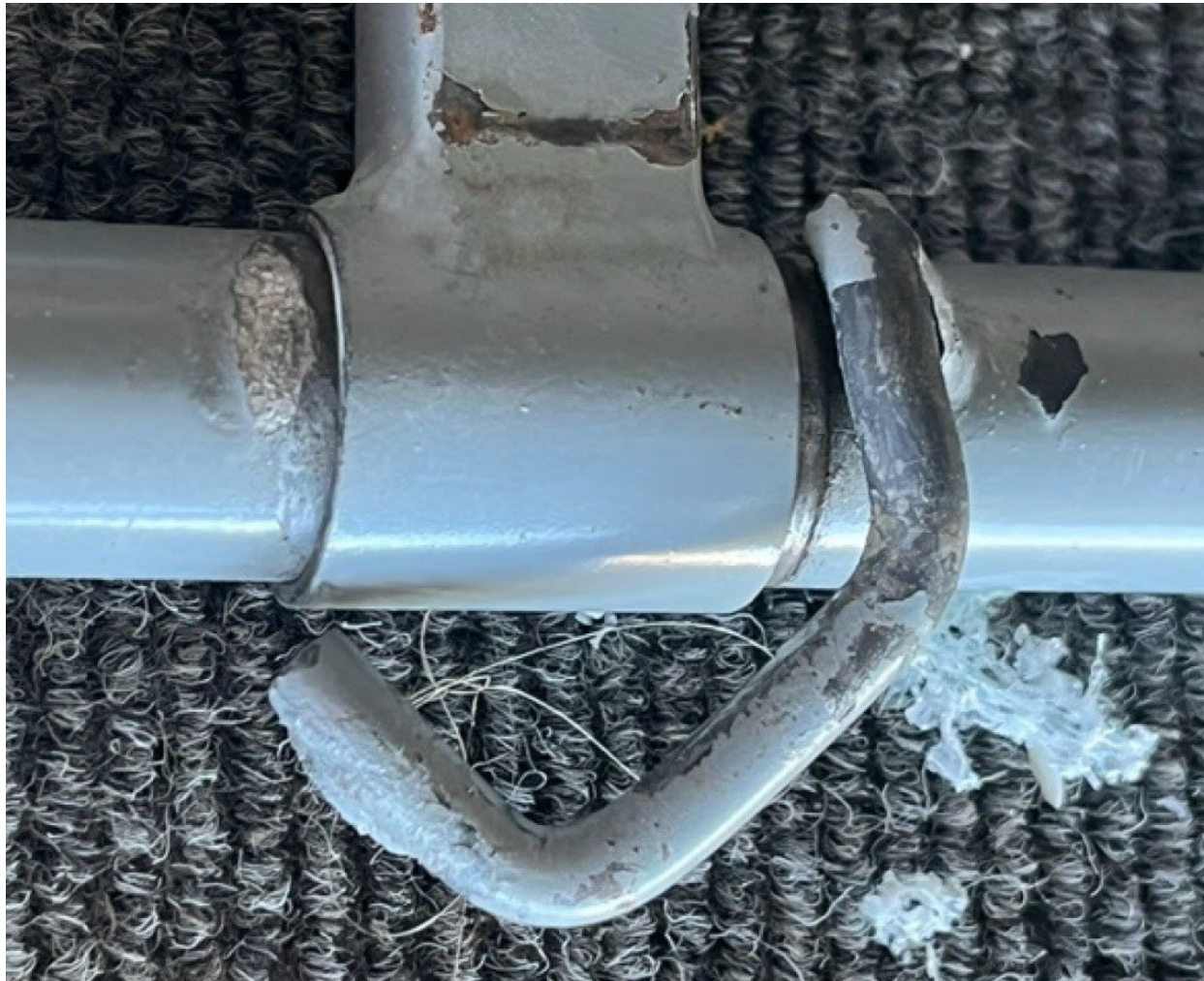
Photograph 7 - Failed weld (Courtesy of FAA)
