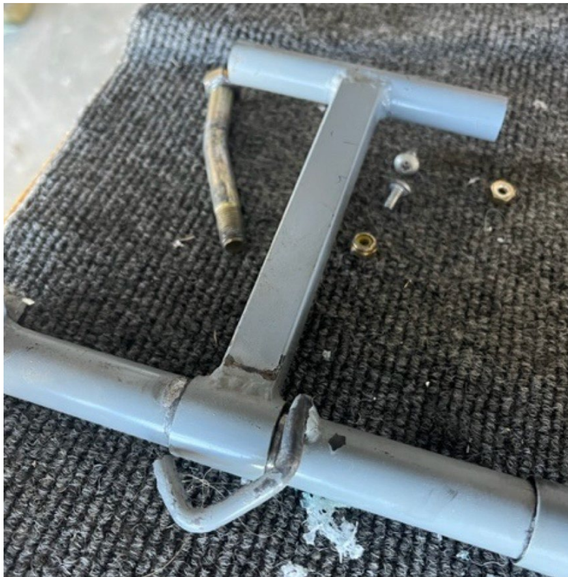
Photograph 10 - Failed weld (Courtesy of FAA)
