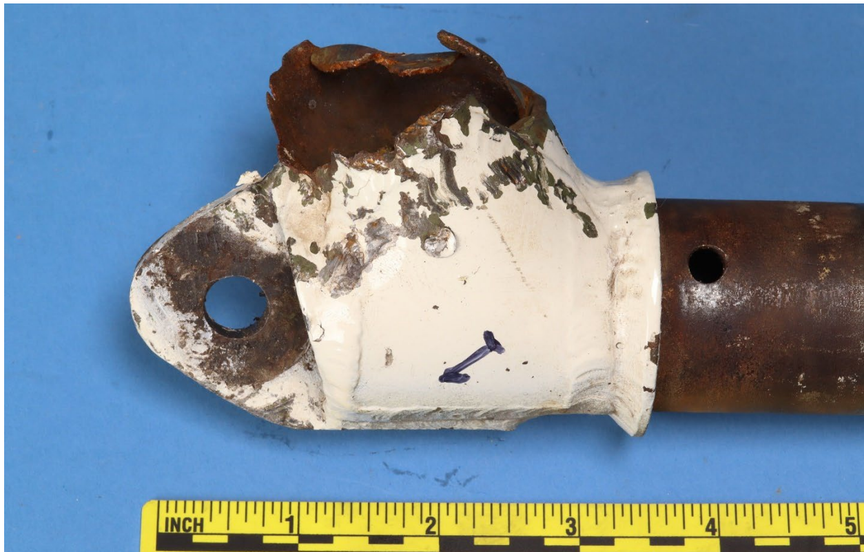
Figure 6. View of the collar side of fracture 1, showing material deformed inward on the far side, and fractures oriented in line with the leg on the near side of the figure.
