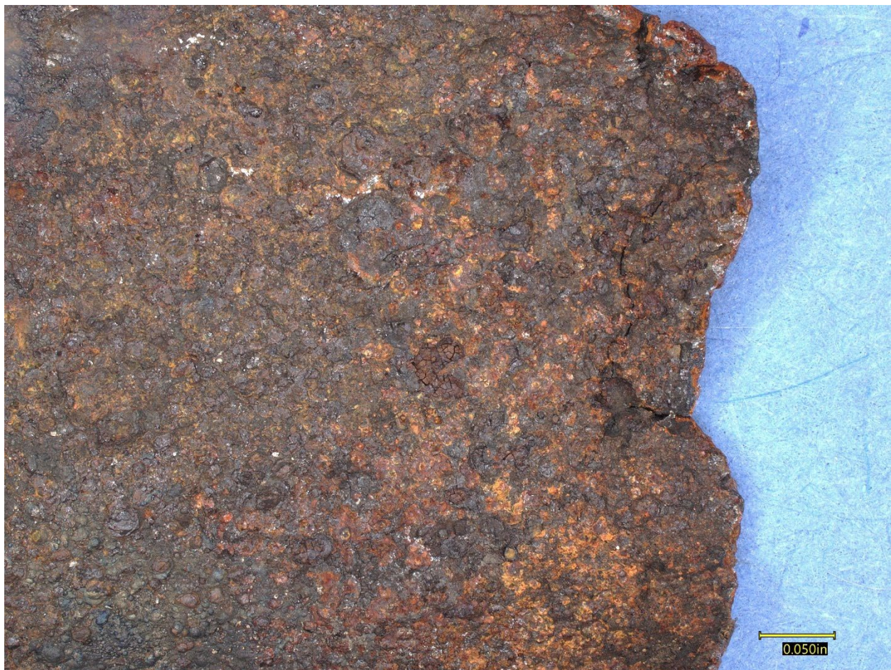
Figure 21. View of the inside surface of the leg tube of the collar (oriented downward in Figure 20).
