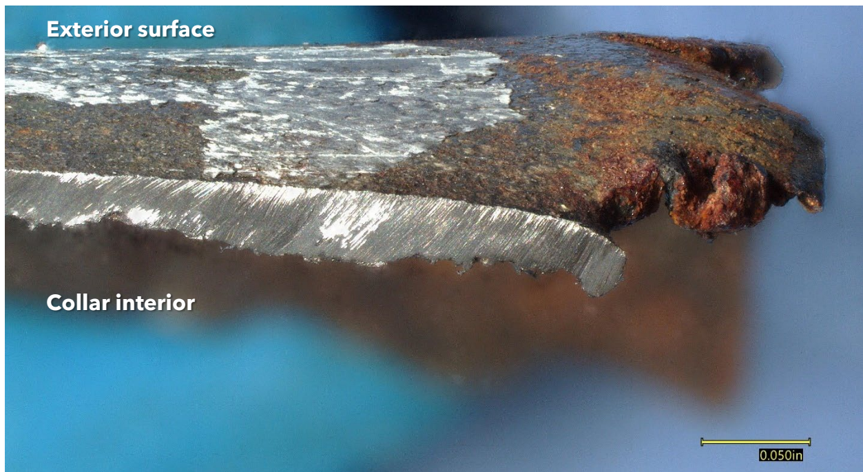
Figure 19. Cross section through the thin fracture surface, viewed from the side.
