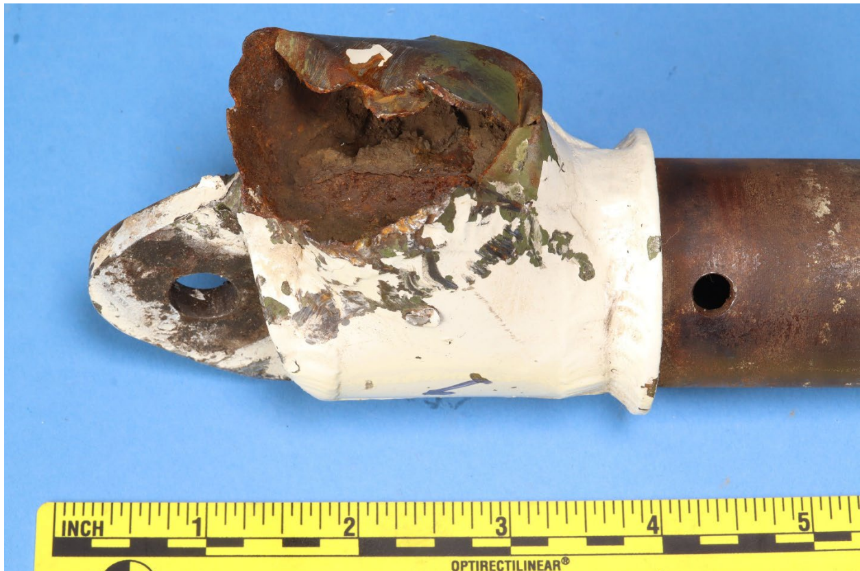
Figure 7. Angled view of Figure 6, showing the deformed side of the collar, and interior corrosion products.
