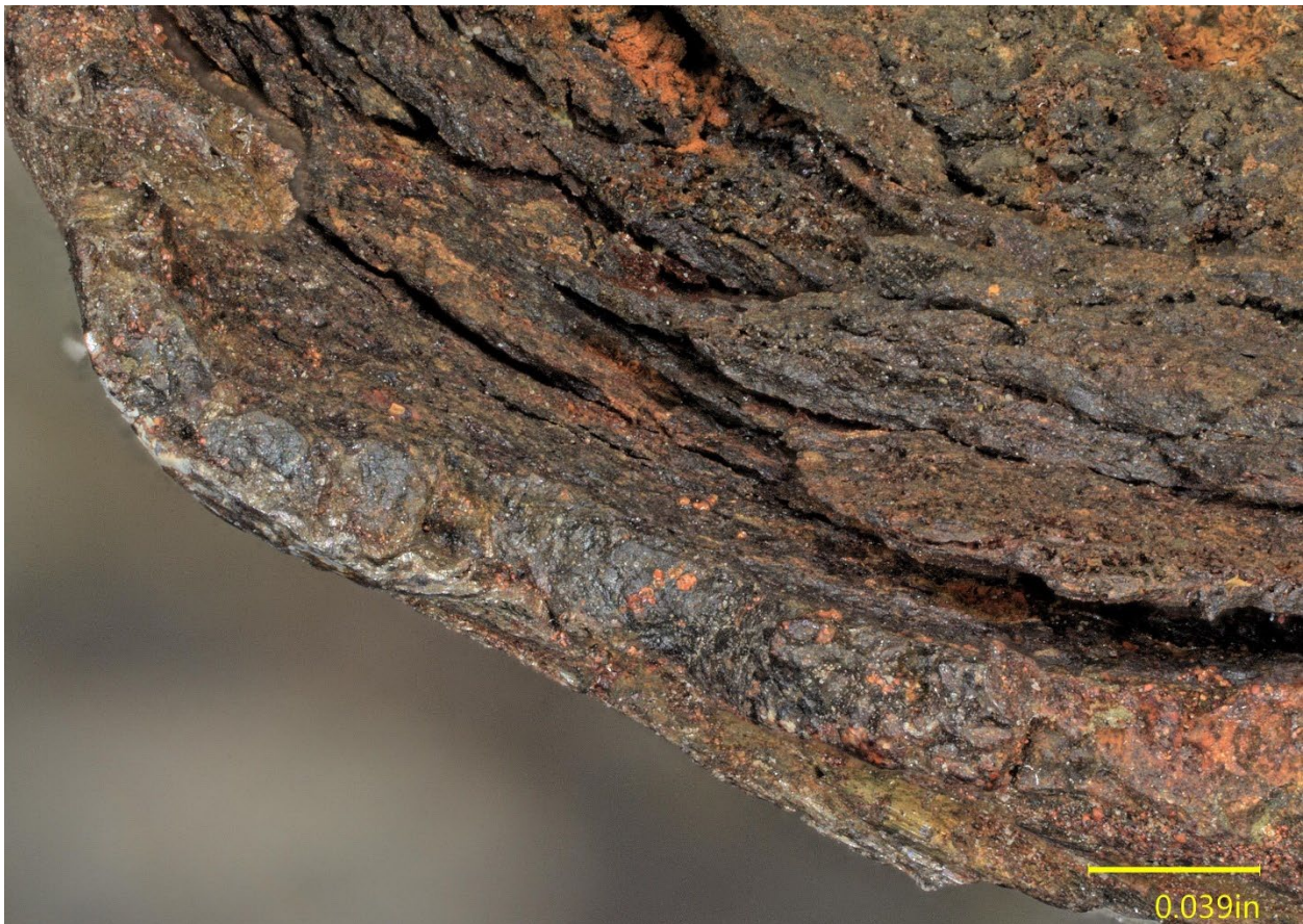
Figure 13. View of a thicker area of the fracture surface, showing layered interior compounds.
