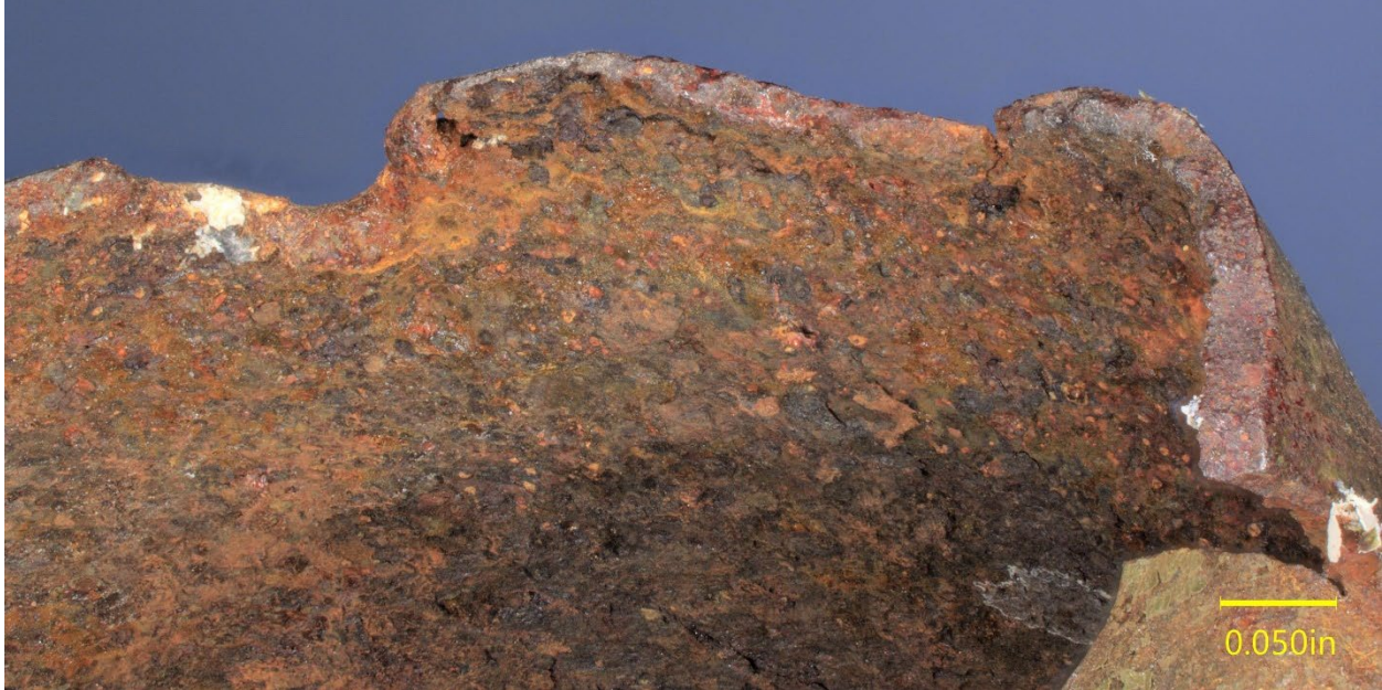
Figure 12. Closer view of the right side of the fracture in Figure 11, showing material thinning.
