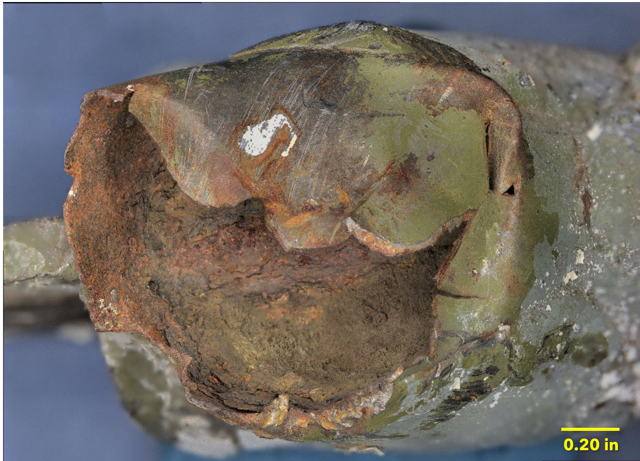
Figure 10. Closer view of the deformed area of the tube fracture near the collar at fracture 1.
