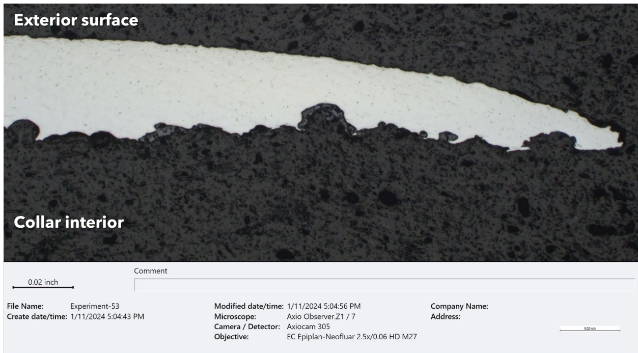
Figure 23. Bright field (BF) optical micrograph of a cross section through the thinnest part of the landing gear leg collar side fracture (~25X, as polished).
