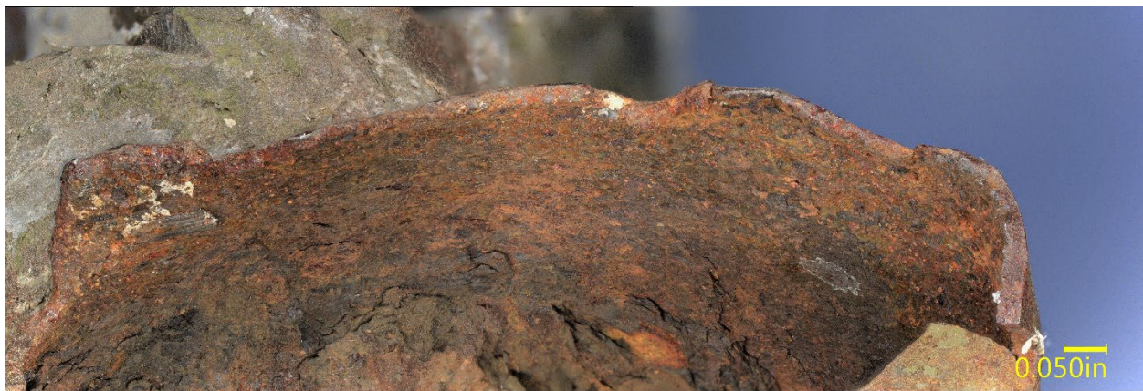
Figure 11. Closer view of the un-deformed portion of the collar fracture surface.
