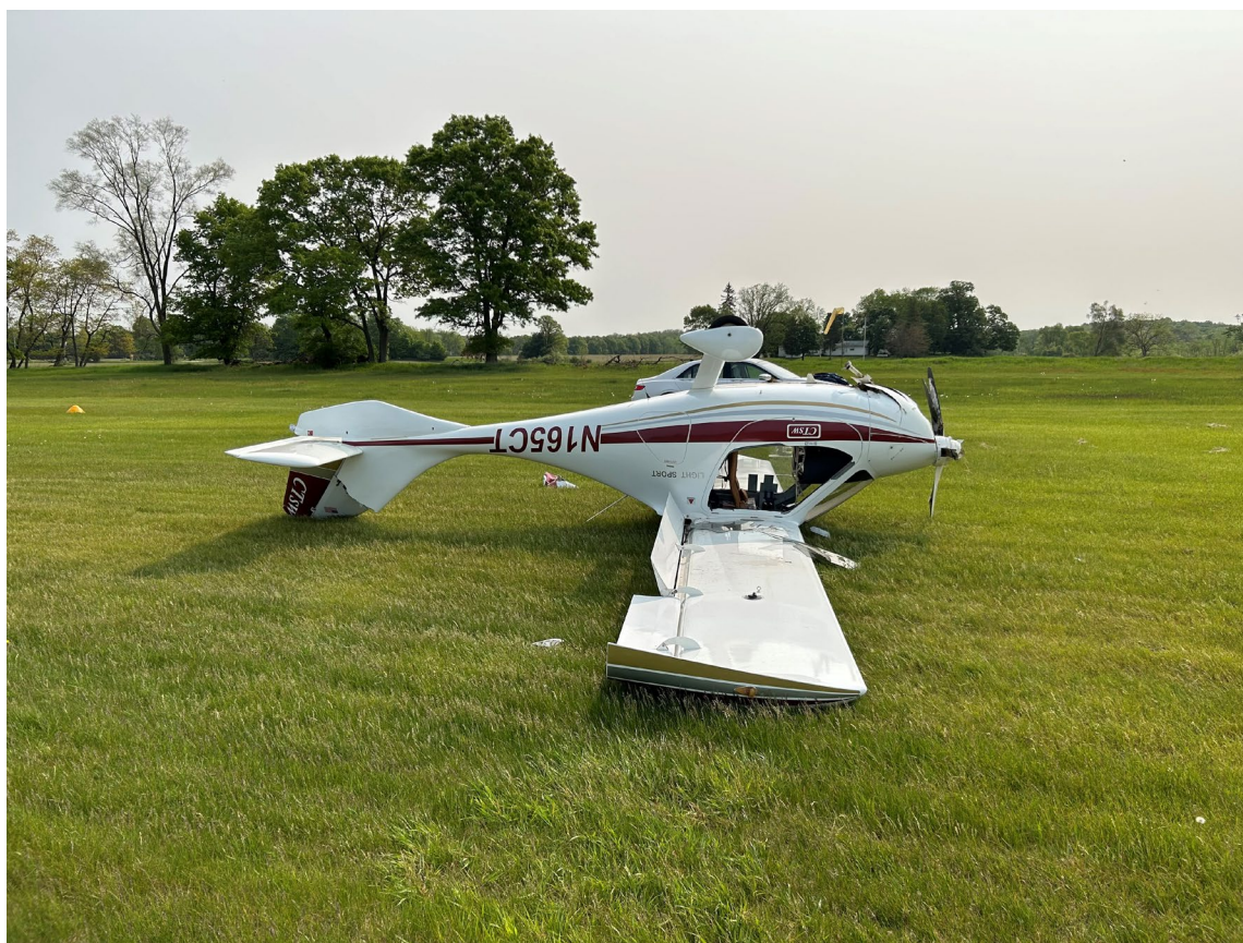
Photograph 1 - Fractured vertical stabilizer (Courtesy of FAA)
