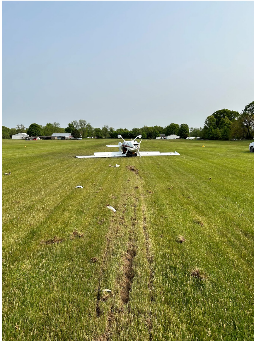
Photograph 3 - Ground scars from landing (Courtesy of FAA)
