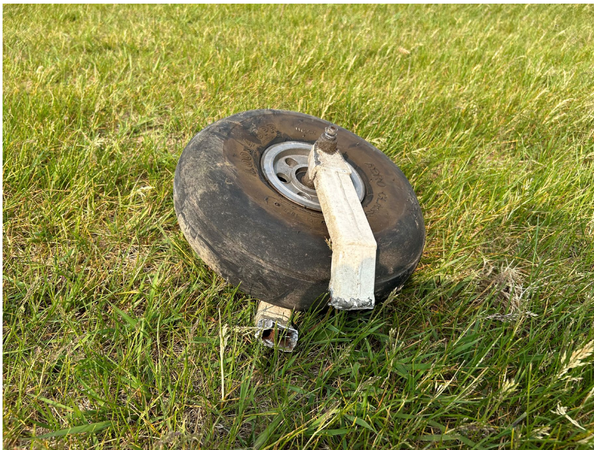
Photograph 4 - Separated section of the nose landing gear (Courtesy of FAA)
