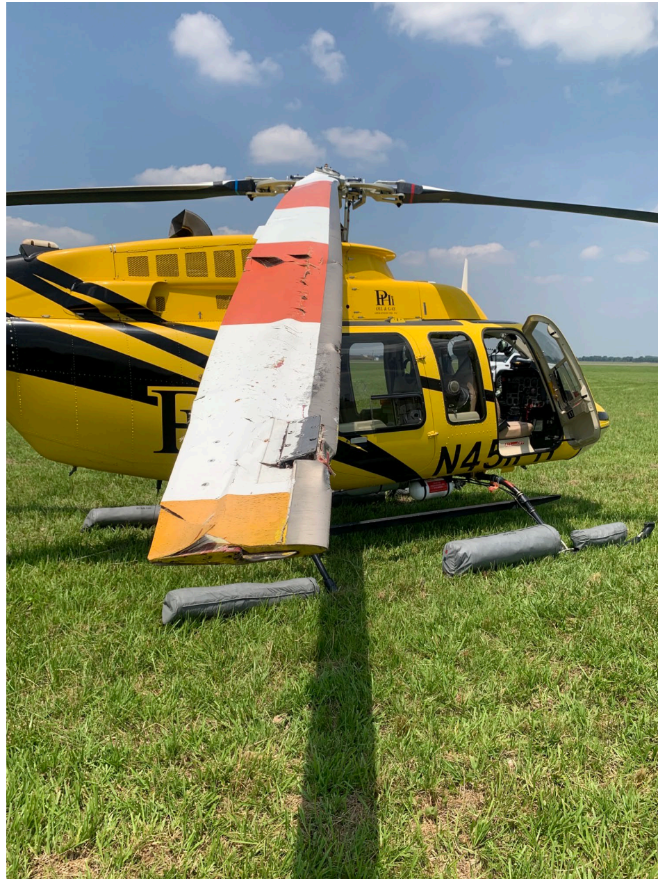
Photo 4 – View of the main rotor blades at the accident site (courtesy of the Federal Aviation Administration).
