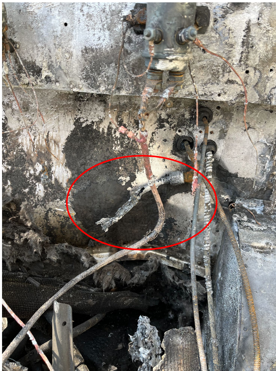
Photo 7 – Melted fuel line (Source: FAA)
