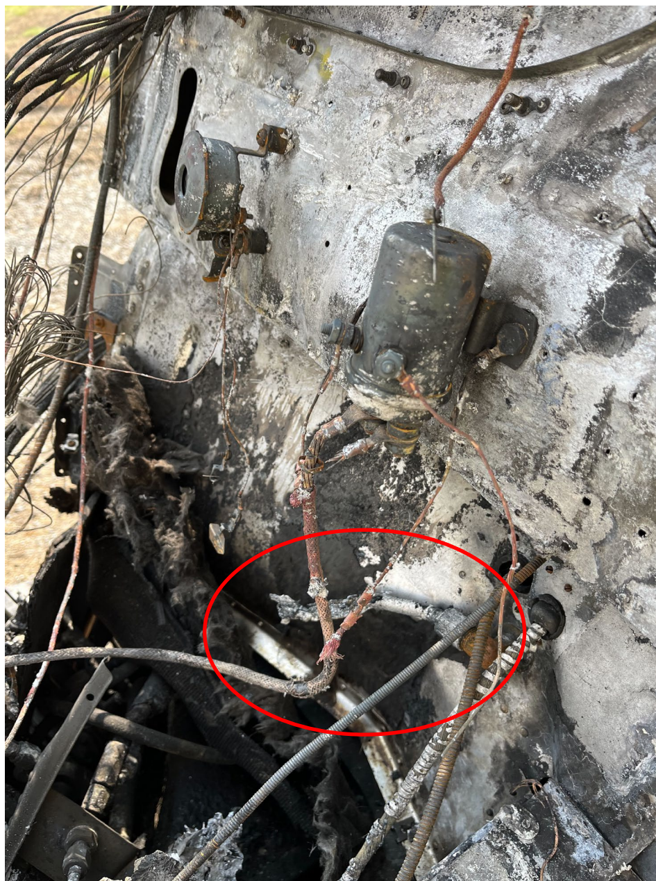
Photo 6 – Melted fuel line (Source: FAA)
