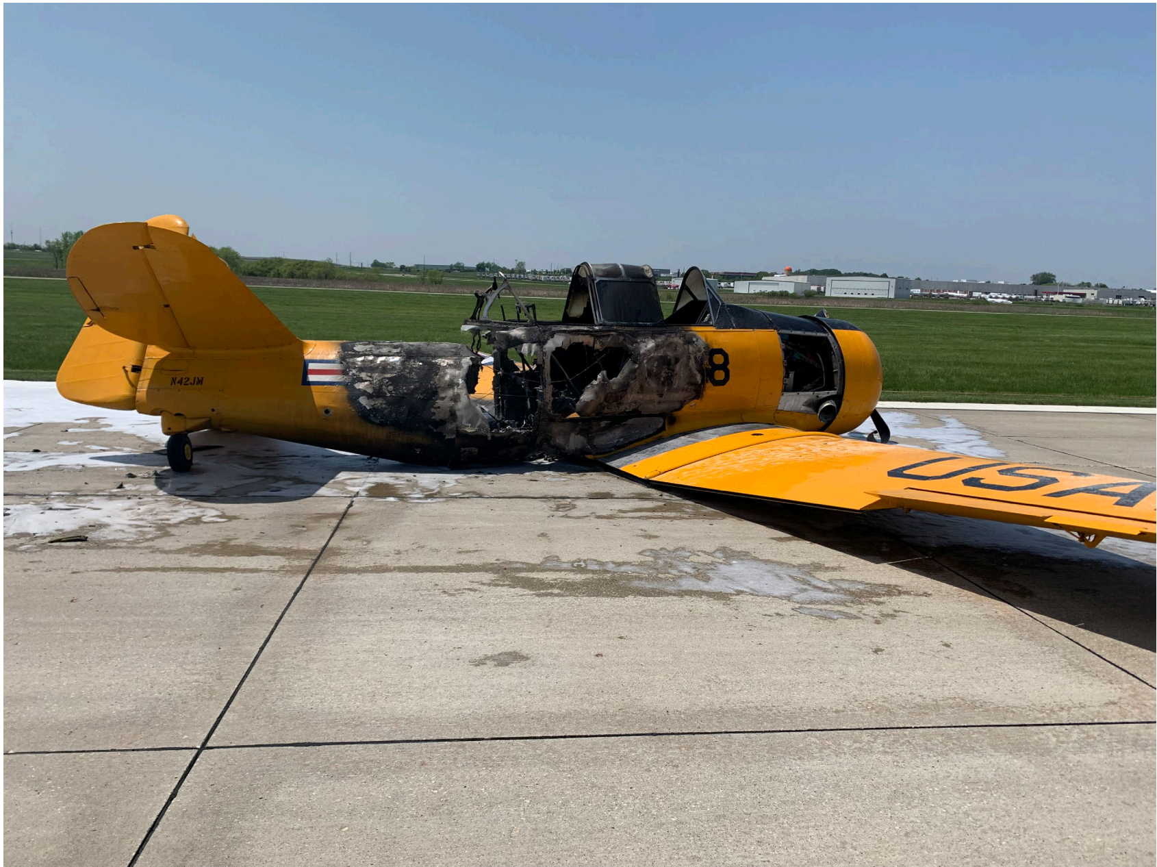
Photo 2 – View of thermal damage to the fuselage, and retracted landing gear (Photo provided by FAA)
