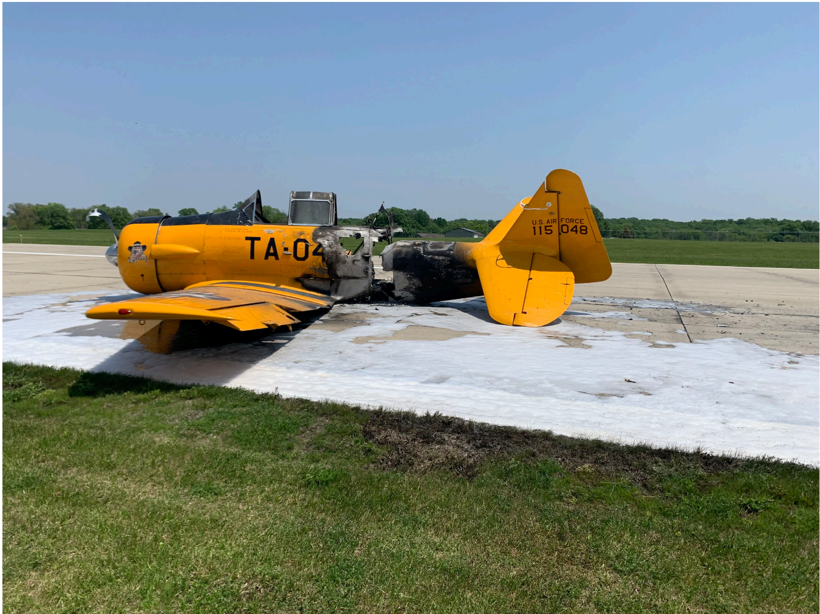
Photo 1 – View of thermal damage to the fuselage and left wing (Photo provided by FAA)
