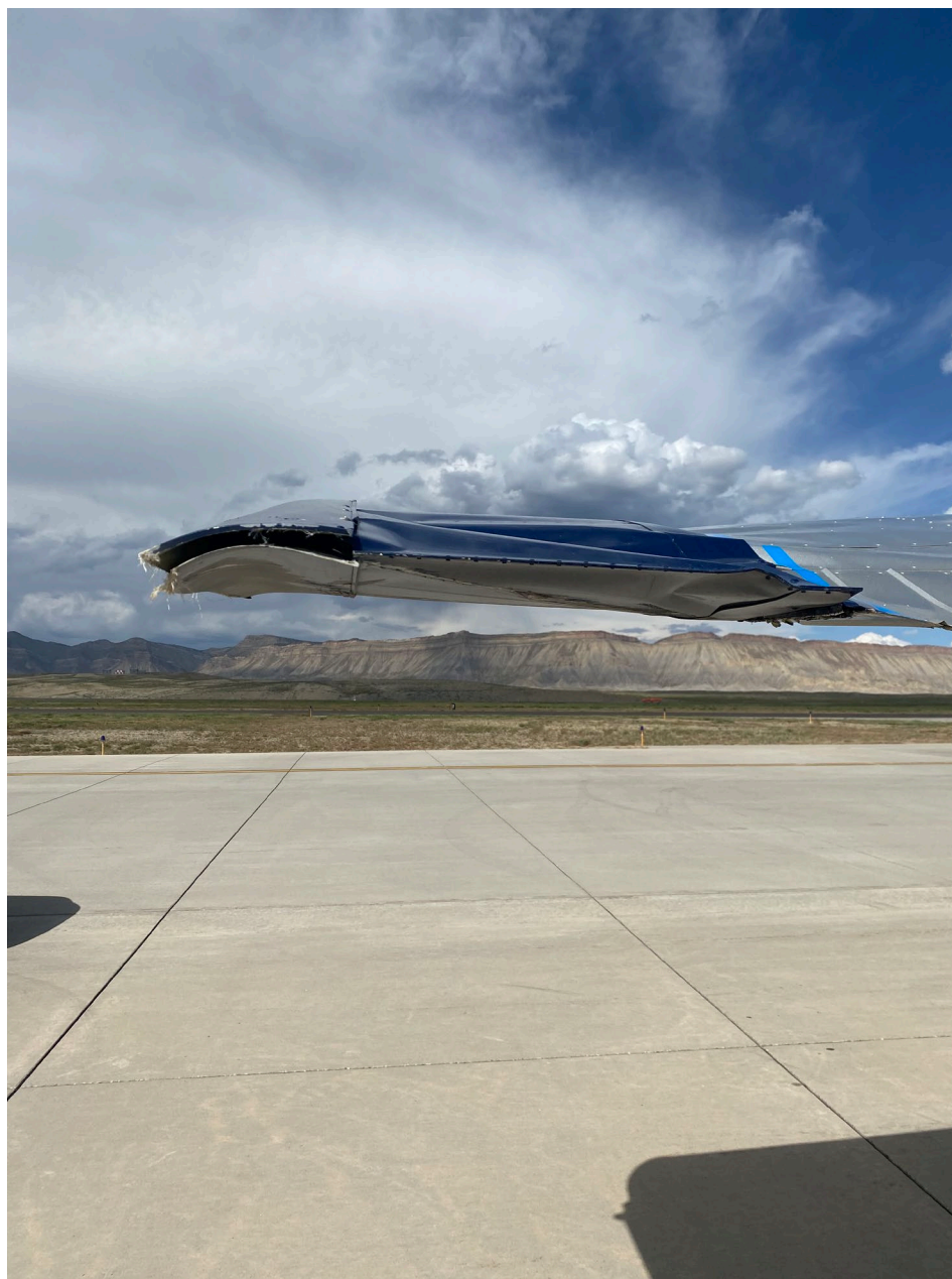
Photo 2 – Accident Airplane Damage to Left Wing (Source: Airplane Owner)
