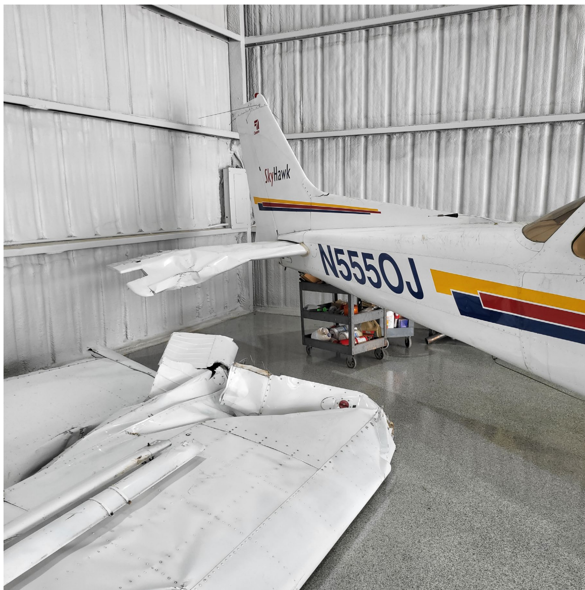
Photograph 2 - Damage to Right Horizontal (Courtesy of FAA)
