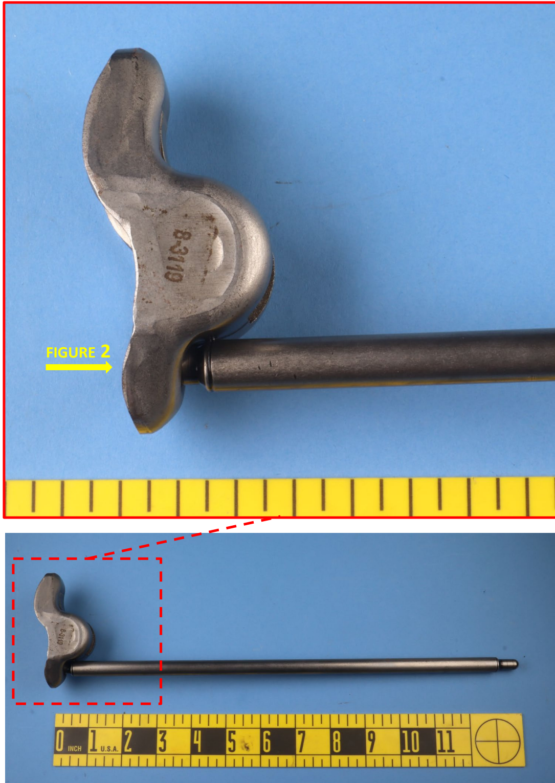
Figure 1. Overall (bottom) and close-up (top) photos showing the stuck together pushrod and rocker arm. A close-up photo showing the inner surface of the rocker arm looking in the direction of the yellow arrow is shown in Figure 2.
