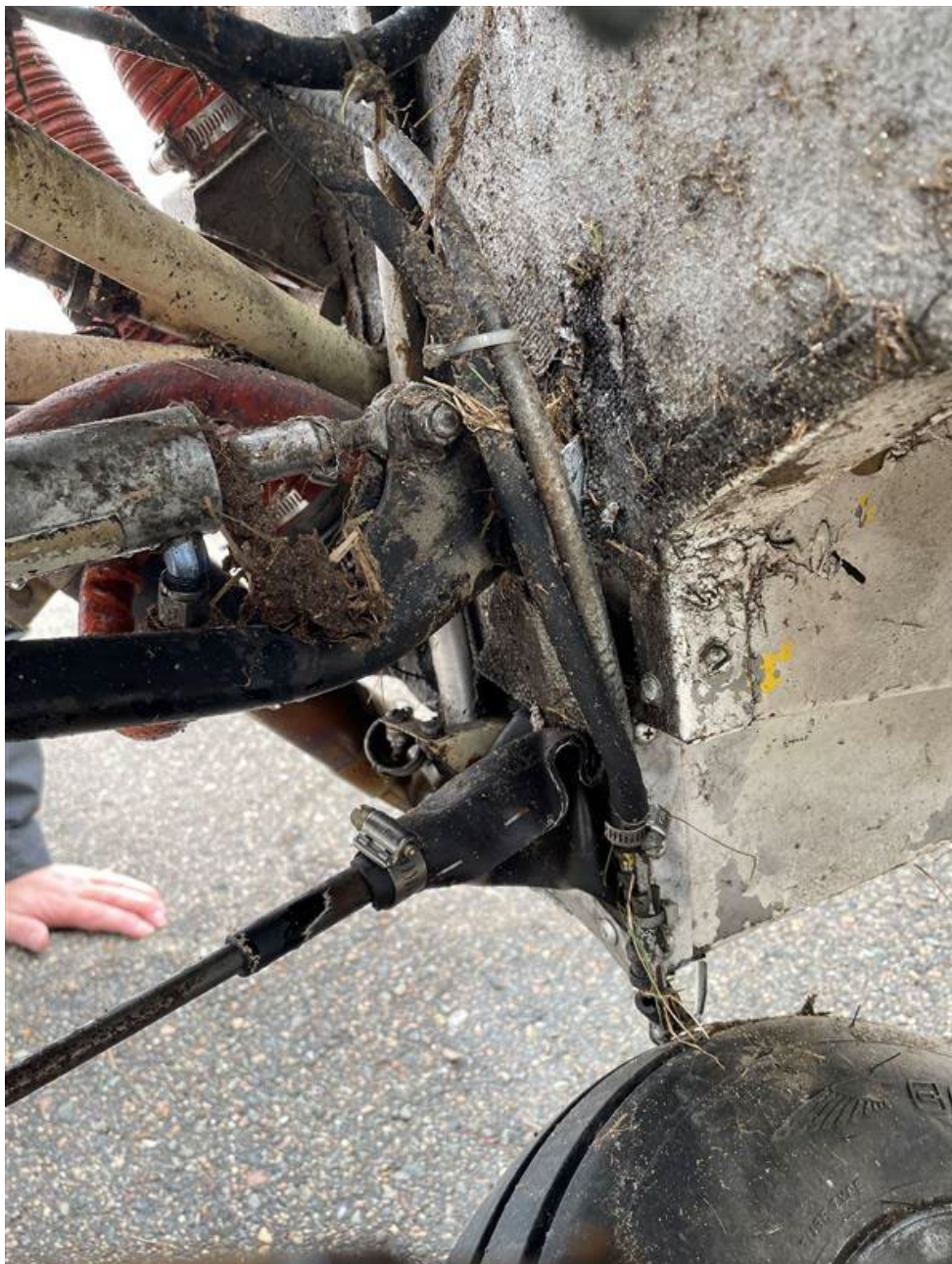
Photo 3 - View of substantially damaged engine mount (Photo Provided by FAA)
