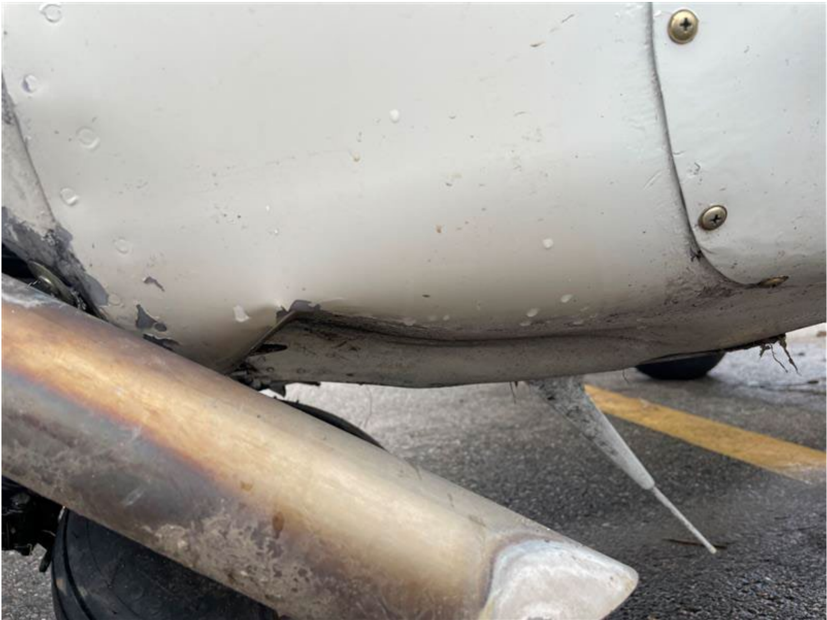
Photo 2 - View of substantially damaged fuselage (Photo Priveded by FAA)
