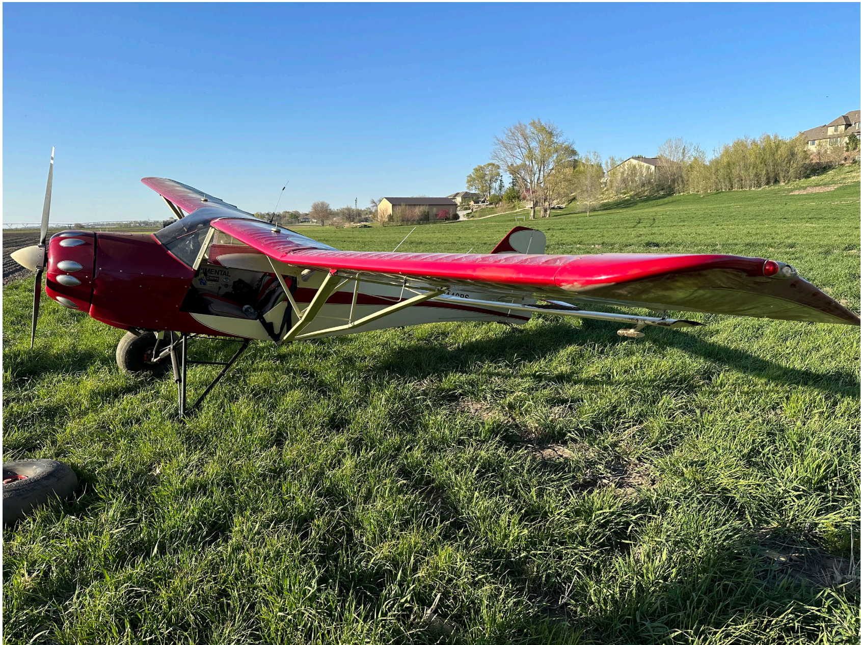
Photo 2 Accident Airplane / Bent Left Wing Spar - (Photo provided by Pilot)
