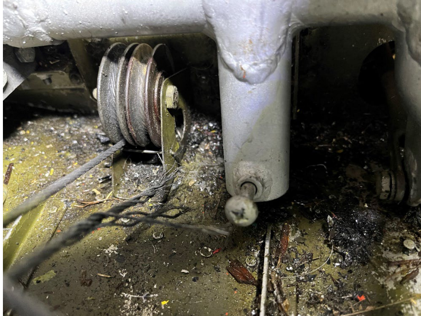
Figure 1. Left Rudder Cable failure point.
