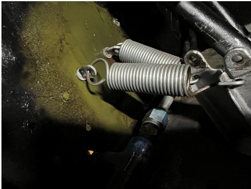
Figure 2. Rudder Return Springs. Left Rudder is the forward spring.
