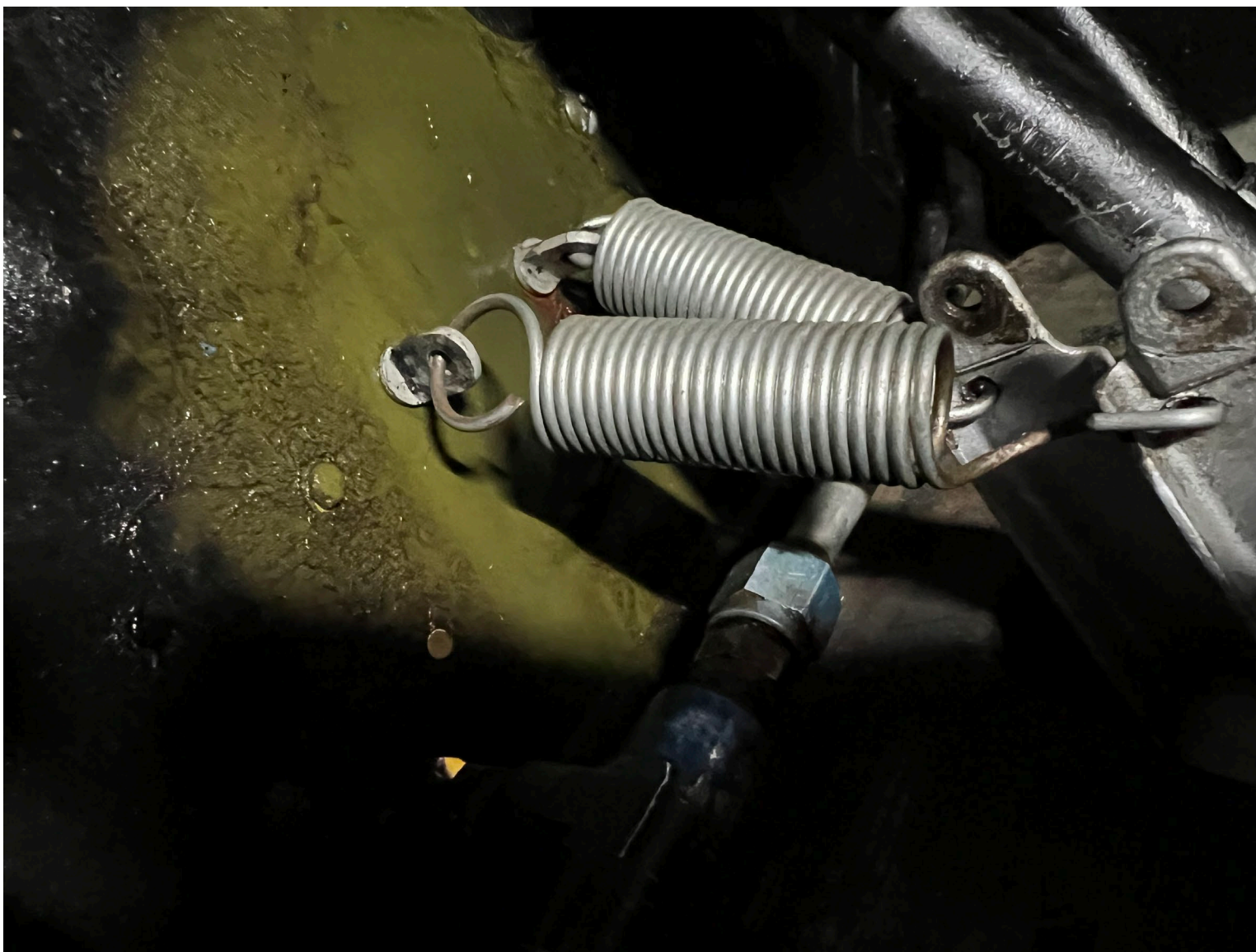
Photograph 3 - Rudder Return Springs with Missing Part on Left Spring (Courtesy of Federal Aviation Administration)
