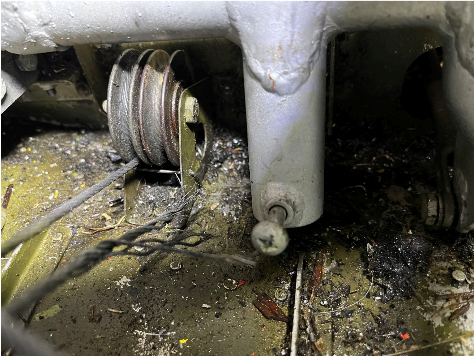
Photograph 2 - Broken Left Rudder Cable at the Pulley (Courtesy of Federal Aviation Administration)
