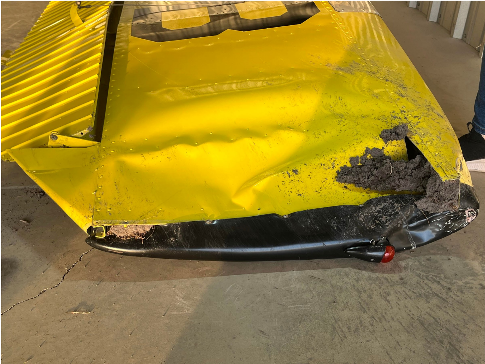
Photograph 4 - Left Wing Damage (Courtesy of airplane owner)
