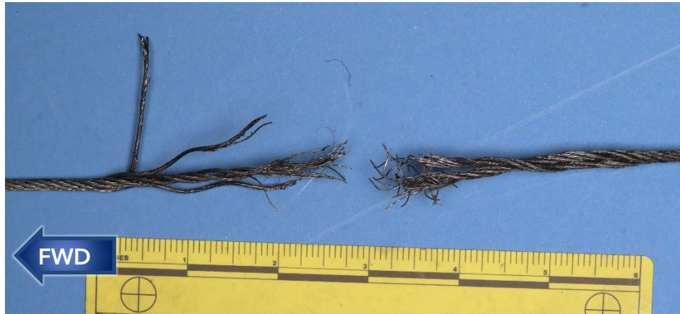
Figure 3. Closer view of the fractured cable ends.
