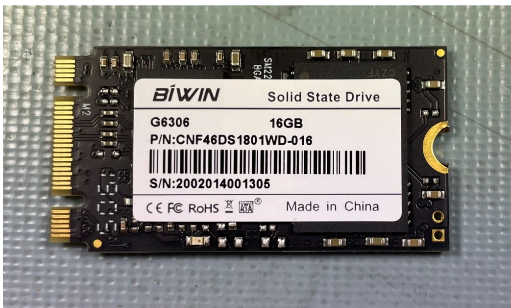
Figure 2. Memory module removed from the recorder.
