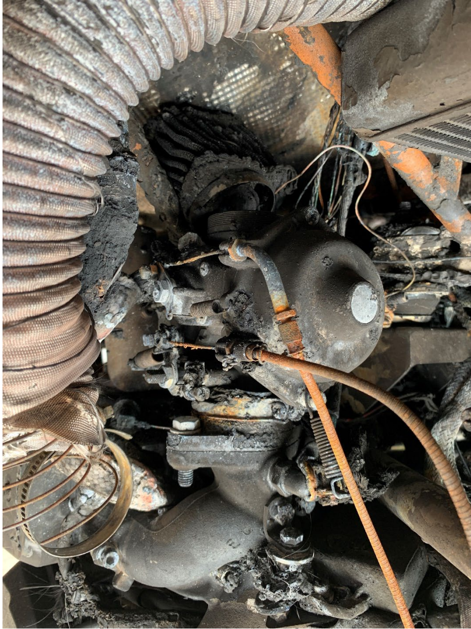
Photo 10: Side View of Right Side Carburetor (Source – NTSB IIC)
