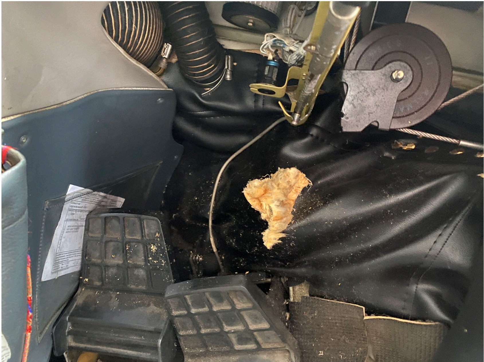
Photo 1 – Damaged floor of fuselage (photo provided by FAA)
