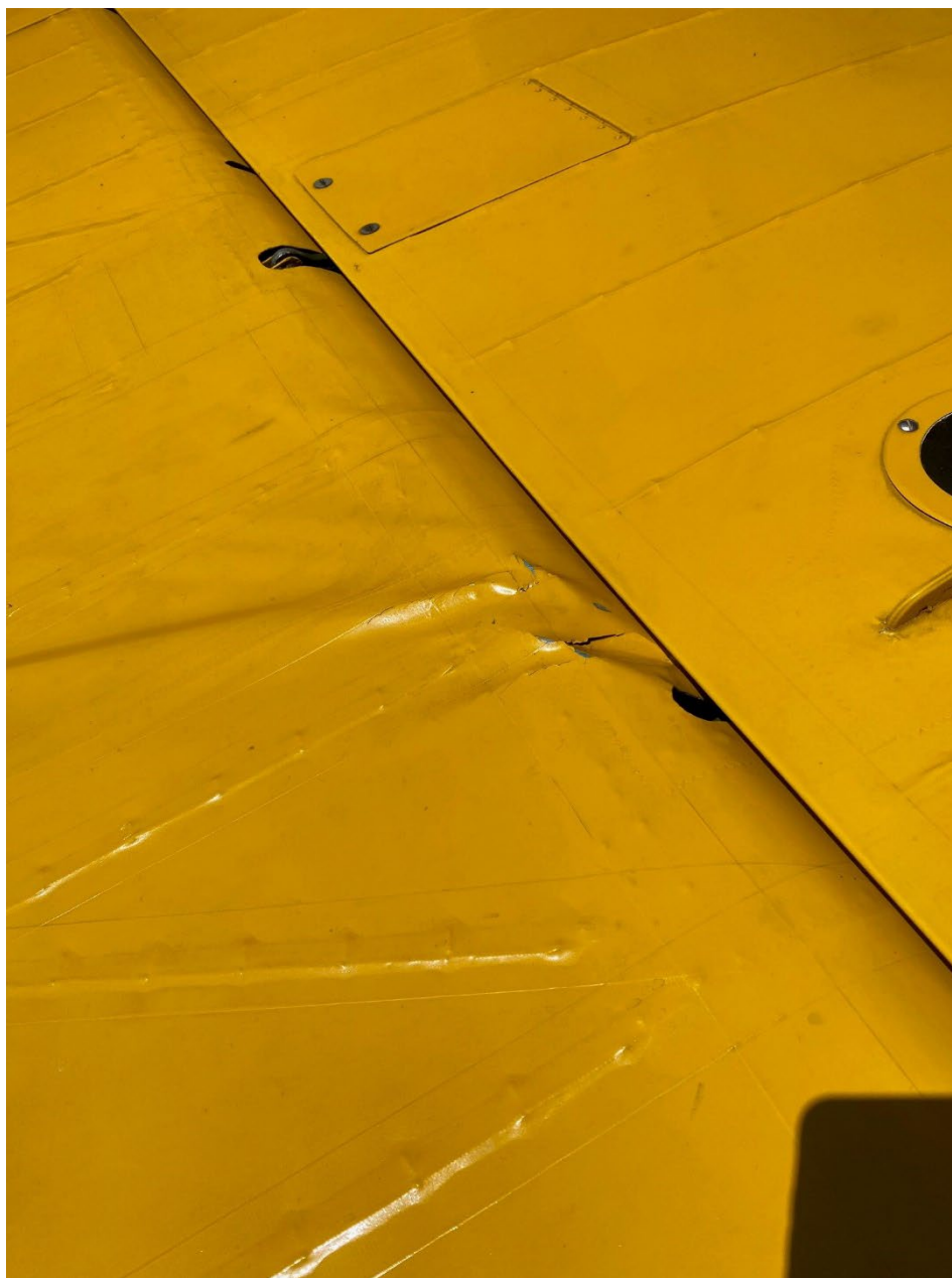
Photo 4 – Close up view of R/H Aileron Leading Edge (EVV Fire/Safety Dept)
