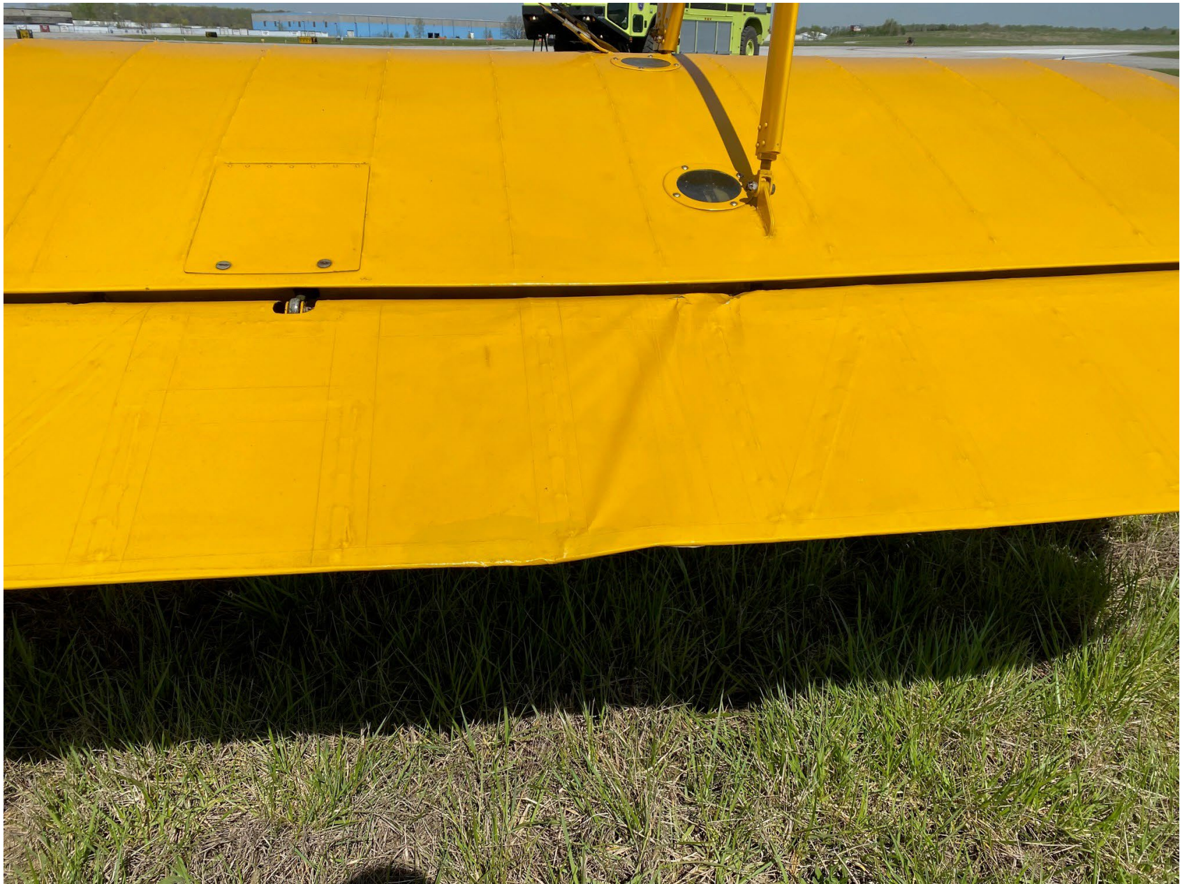
Photo 3 – View of Damage to R/H Aileron (EVV Fire/Safety Dept)
