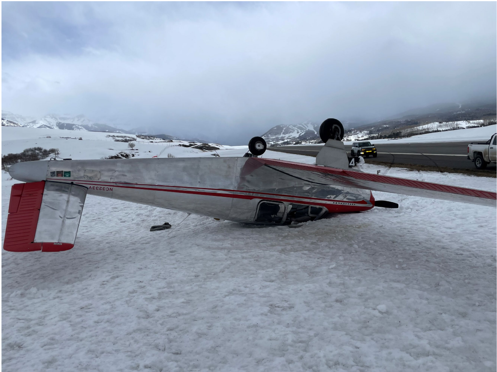
Photo 3: Accident airplane with damage to the V-tail – (Photo provided by the Airport Manager)
