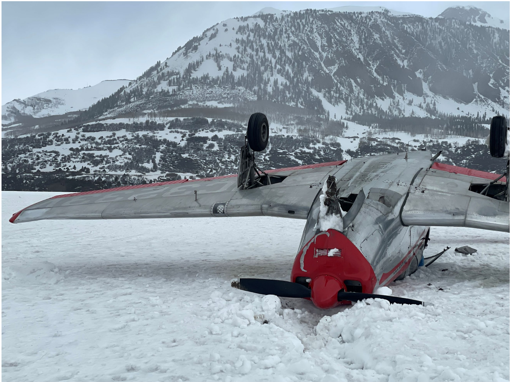
Photo 2: Accident airplane with damage to the left wing – (Photo provided by the Airport Manager)
