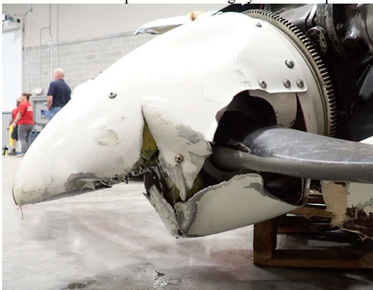
Photo # 2 – Bottom haft of spinner indicating cylinder and piston crushed aft
