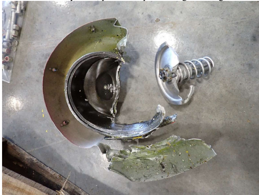
Photo #3 – Cylinder, piston and pitch change rod fragment
