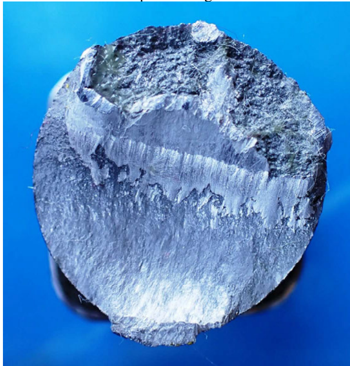
Photo #12 – Blade #1 pitch change knob fracture surface
