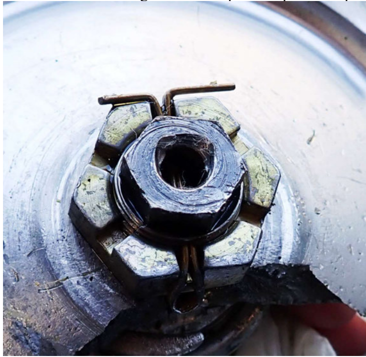
Photo #15 - Pitch change rod at low pitch stop contact point
