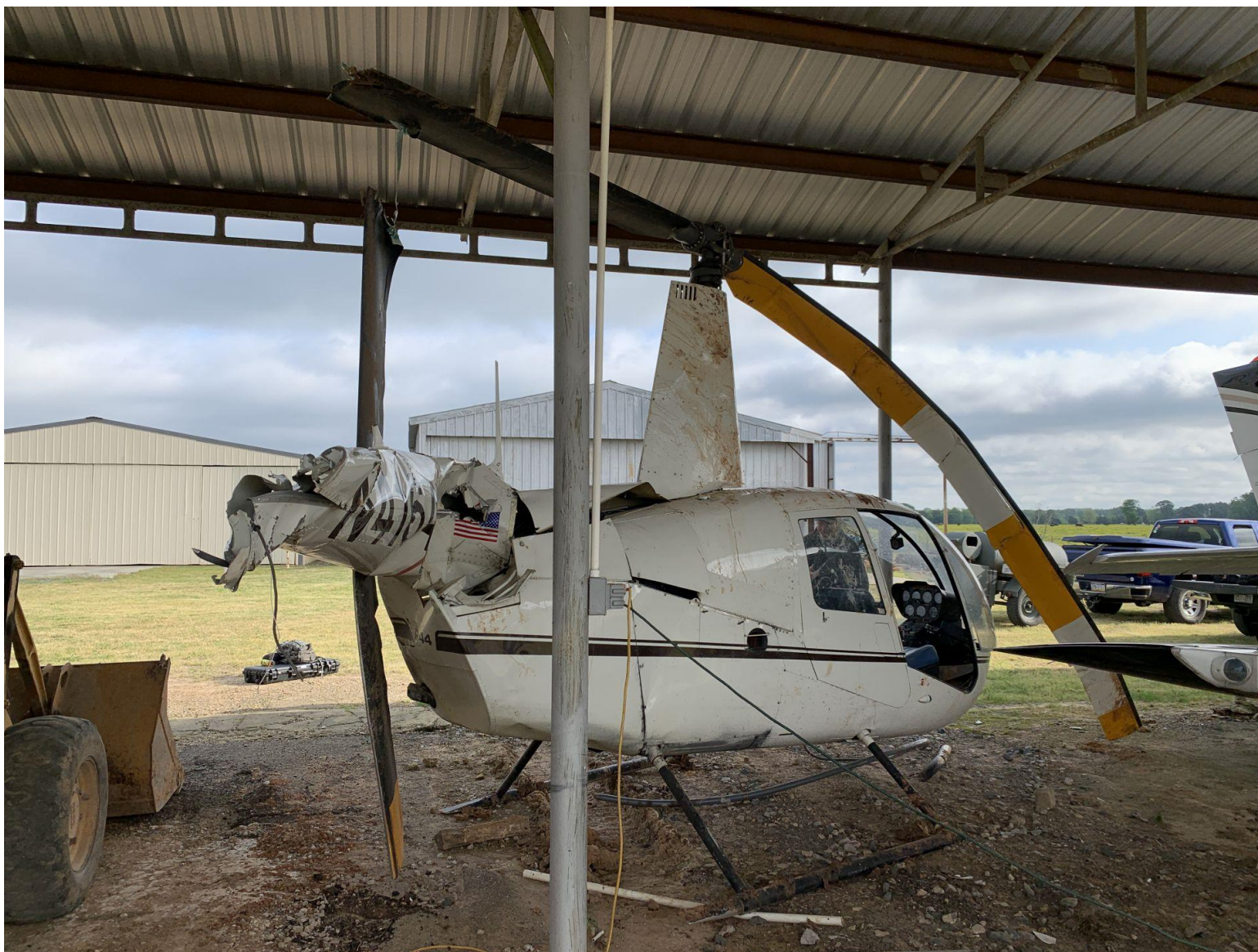
Photograph 6 - Fuselage (NTSB Photo)
