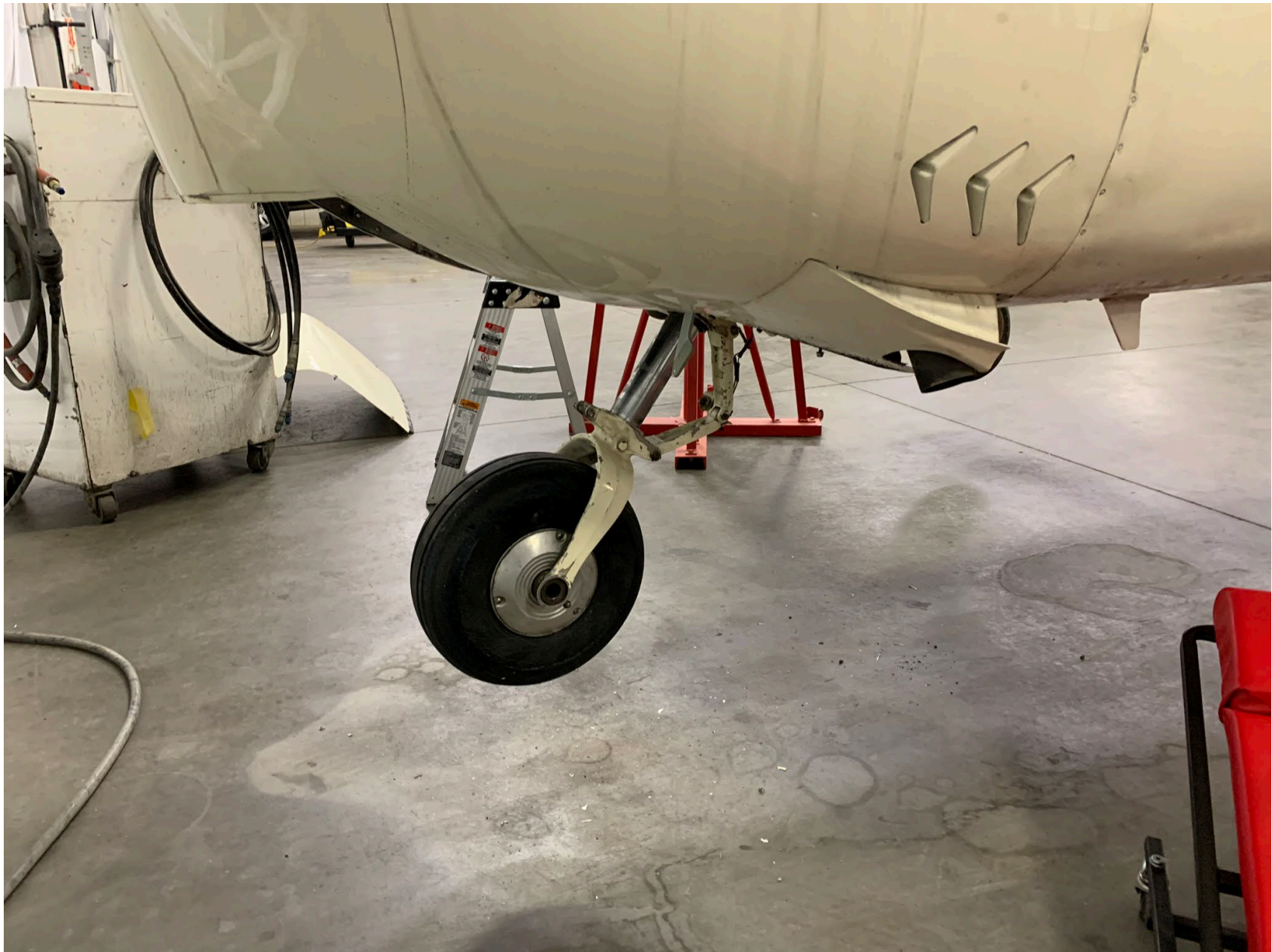
Photo 1 – Nose gear folded forward
