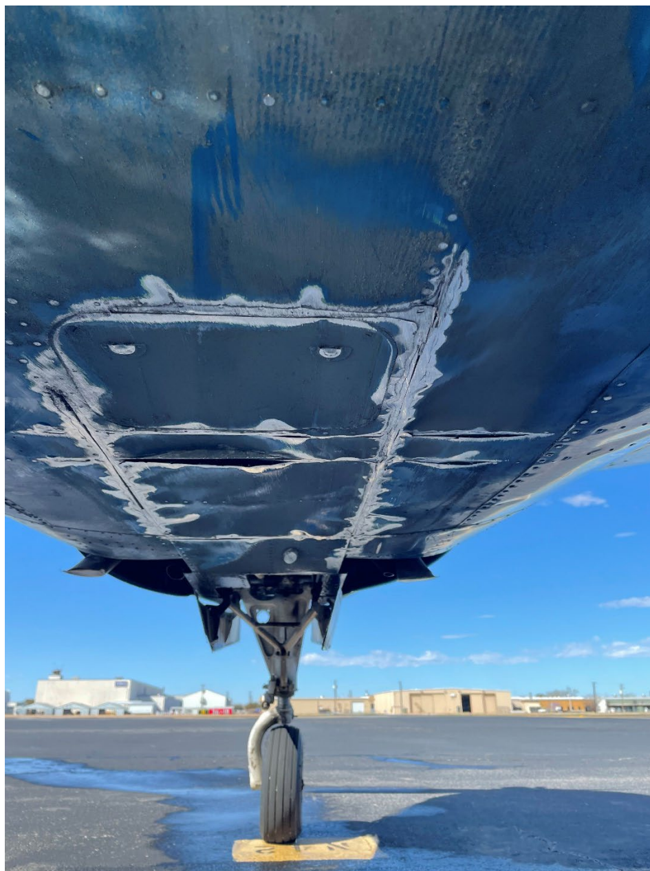
Photo 1 – Substantial Damage to Panels on Belly of Airplane (Photo Provided by FAA)
