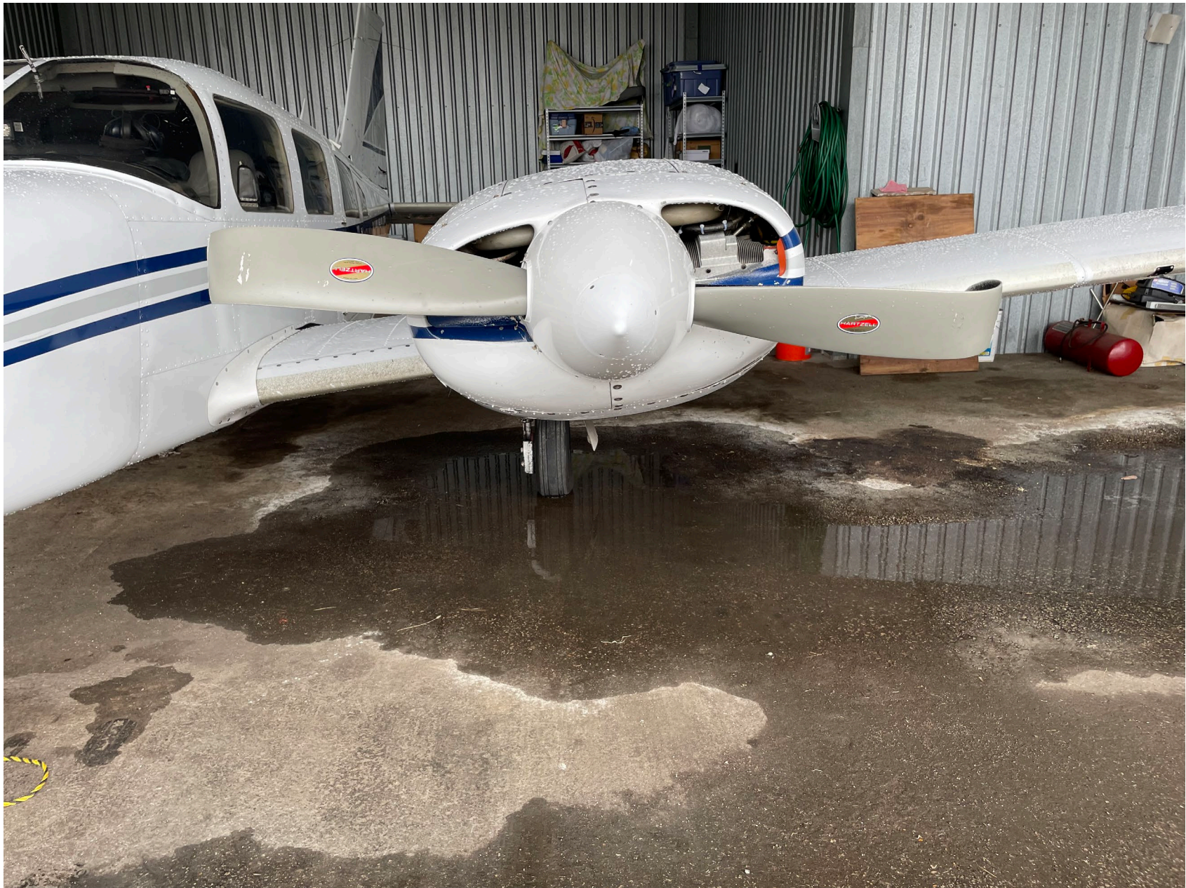
Photo 3: Accident Airplane / Left engine and propeller damage – (Photo provided by the FAA)
