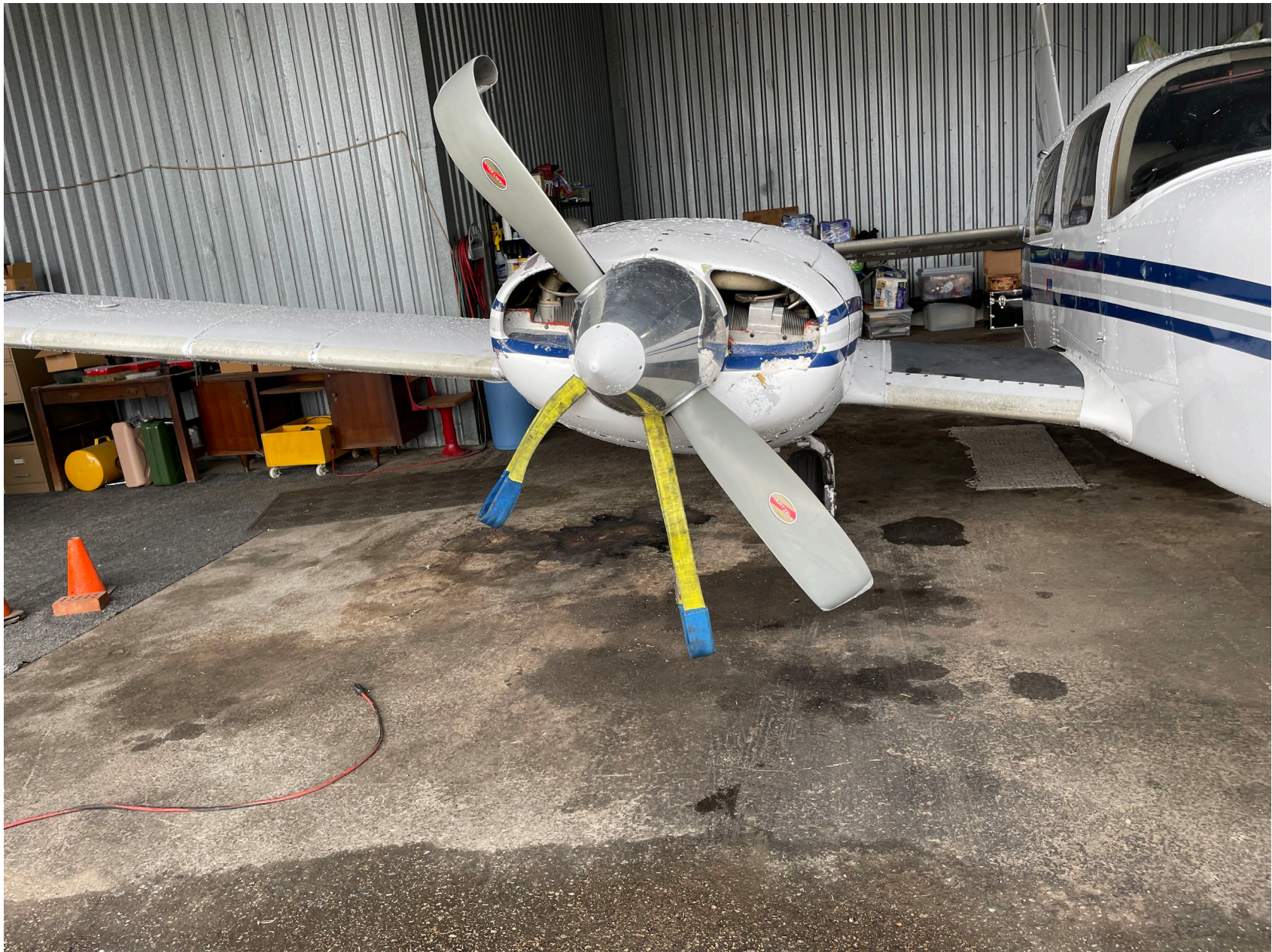
Photo 2: Accident Airplane / Right engine and propeller damage – (Photo provided by the FAA)
