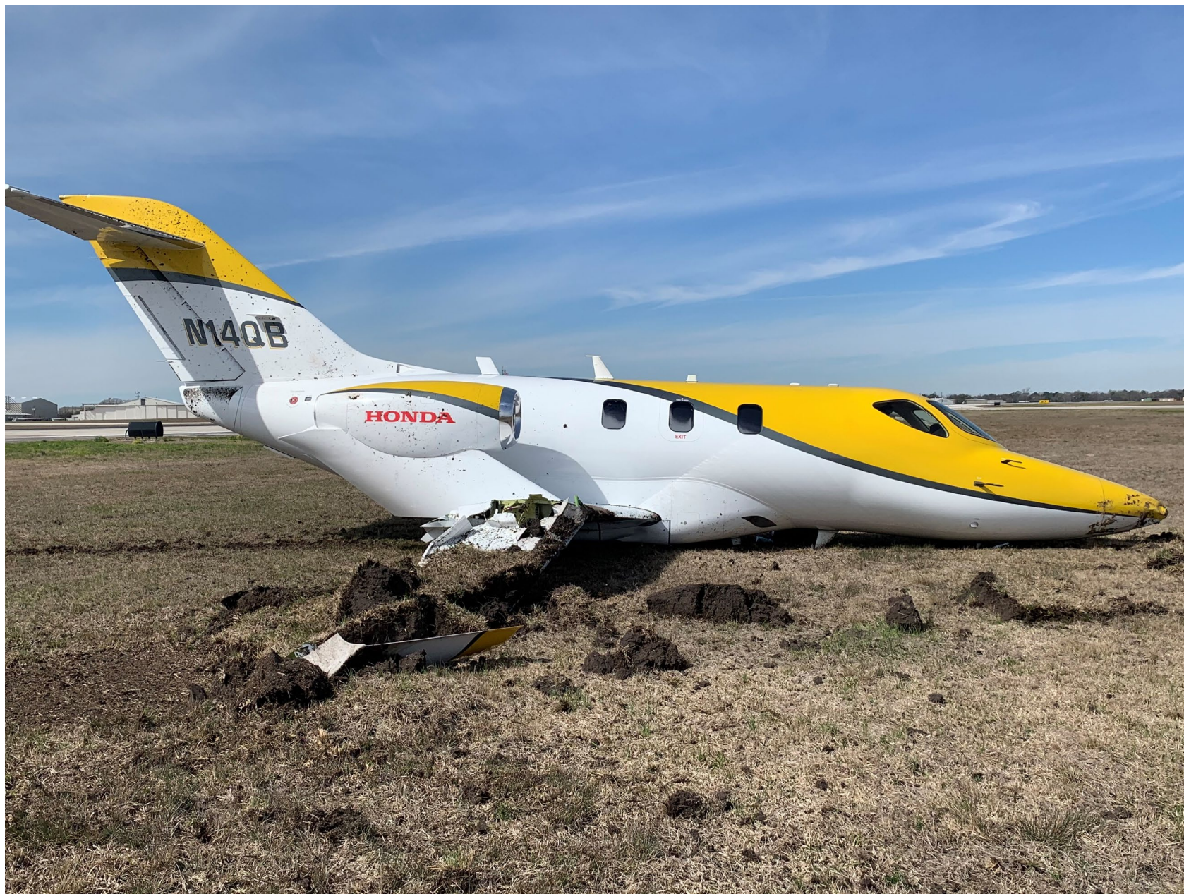
Photo 1: Accident airplane / Damage to the right wing – (Photo provided by FAA)
