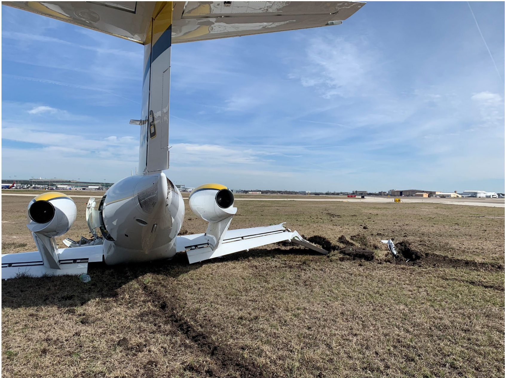
Photo 2: Accident airplane / From the rear with damage to the right wing – (Photo provided by FAA)
