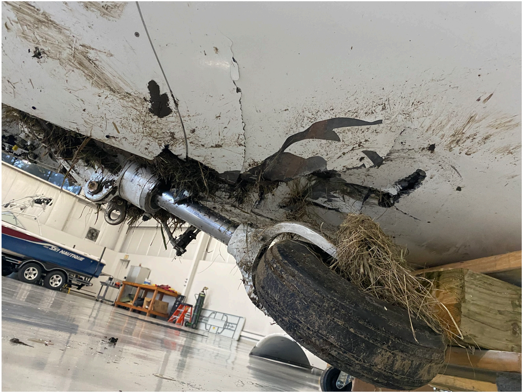
Photo 2 – Forward Fuselage Composite Damage (Source: Airplane Manufacturer)
