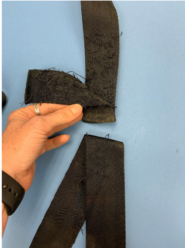
Figure 11. Bellanca Aircraft 7ACA, N9111L pilot's shoulder harness showing stitching failure at the "y" junction.
