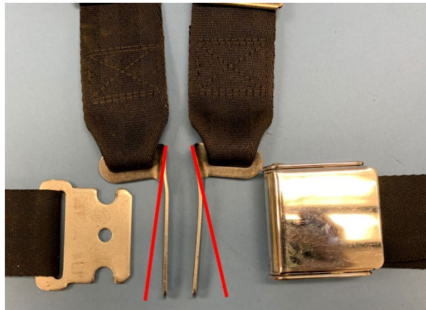
Figure 12. Bent shoulder harness fittings from the accident pilot's restraints. (Red lines indicate approximate normal orientation.)
