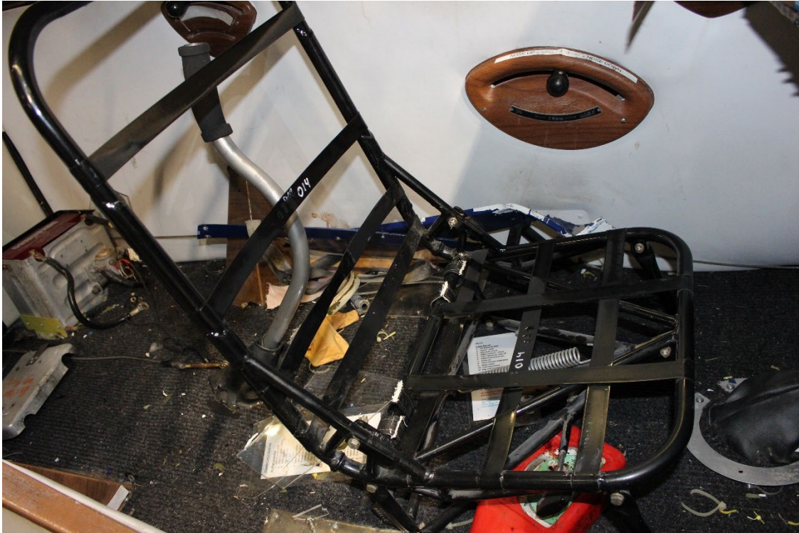
Figure 7. Pilot seat frame with cushions removed.
