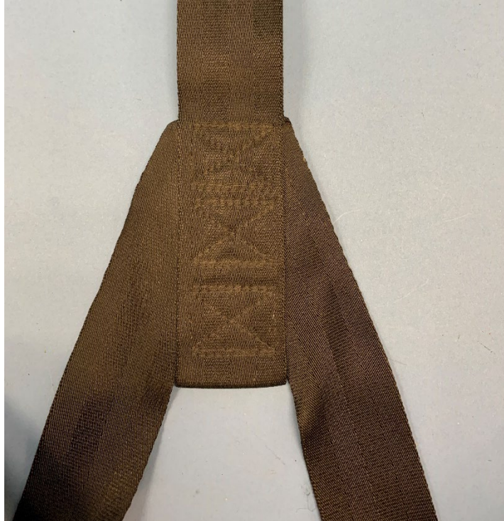
Figure 9. Rear seat belt showing the yoke of the shoulder belt.
