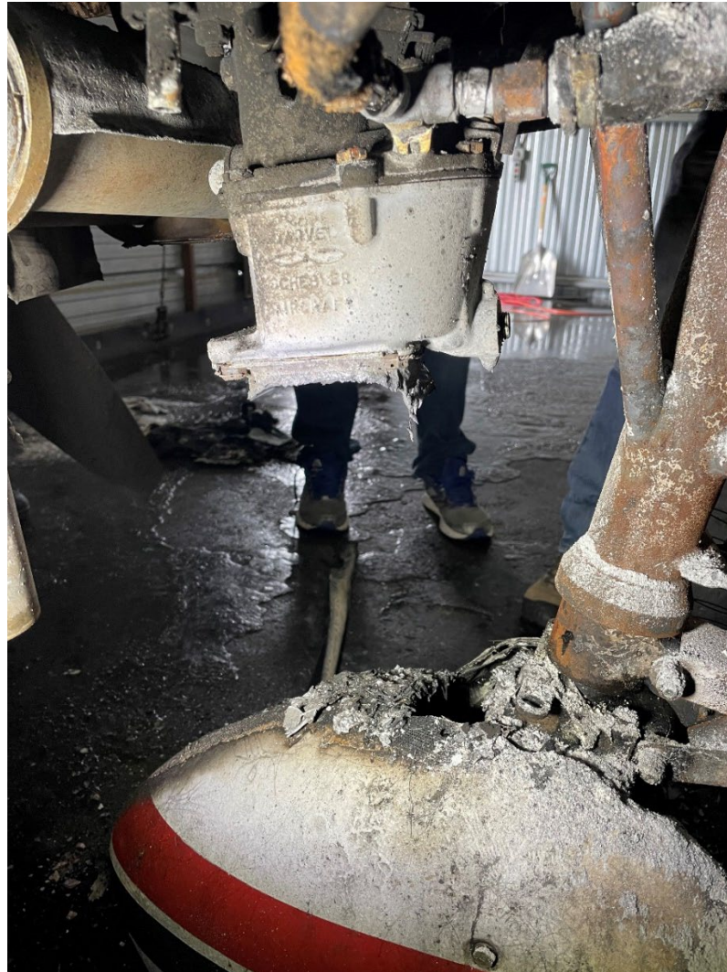
Photograph 6 - Nose Landing Gear and Carburetor Bowl (Courtesy of Federal Aviation Administration)
