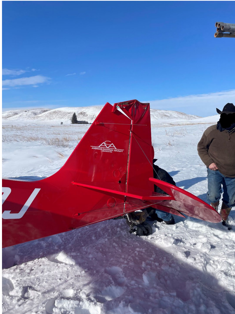
Photo 2 – Accident Airplane – Vertical Stabilizer Damage (Source: Federal Aviation Administration)
