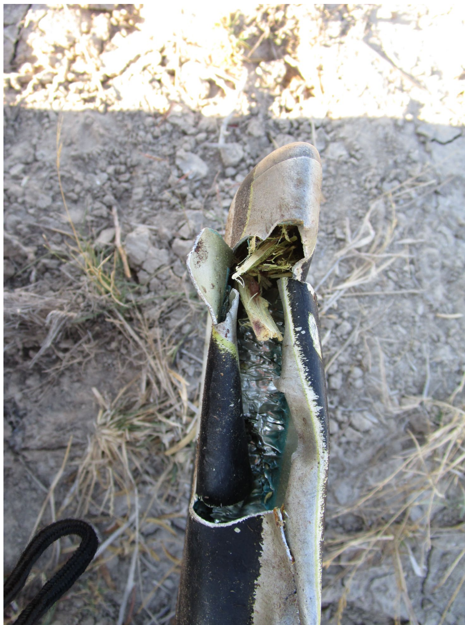
Photo 3 – Tail Rotor with Tree Debris (Courtesy of FAA)
