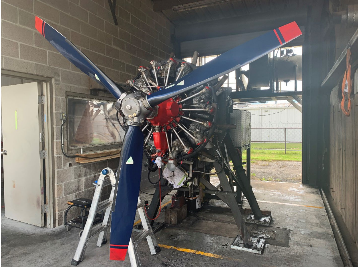
Figure 1. Engine mounted in test cell
