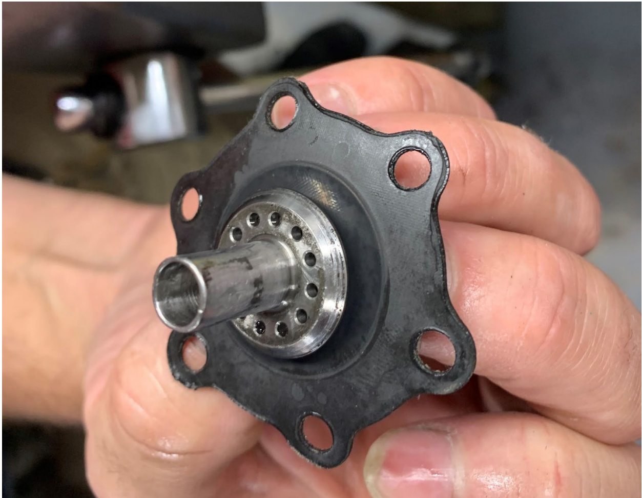
Figure 2. Pressure relief valve with diaphragm
