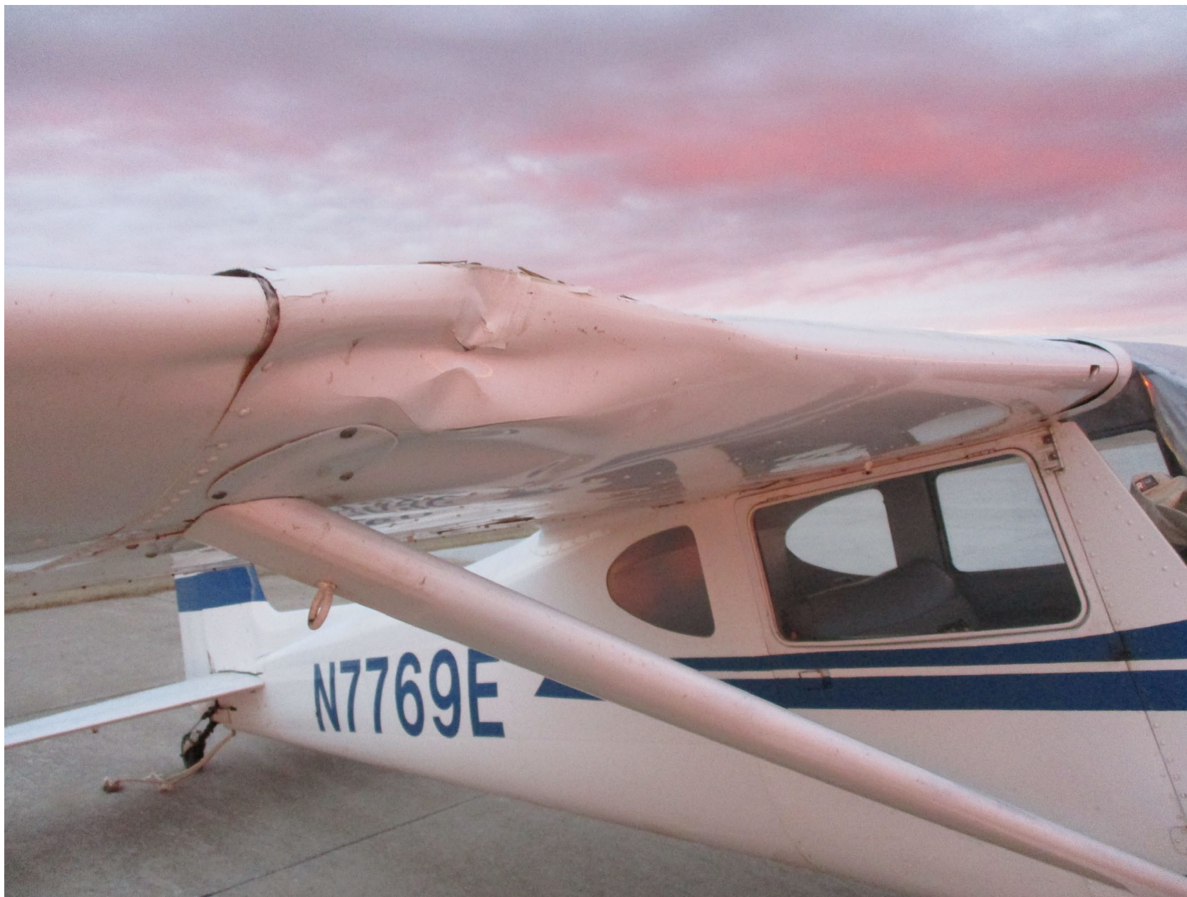
Photo 1 – Crushed Right Wing (Provided by FAA)
