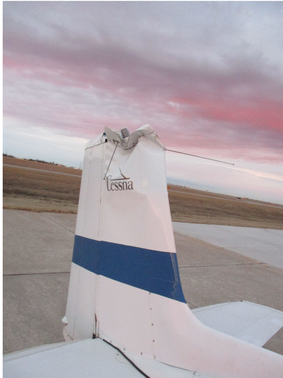
Photo 3 - Crushed Vertical Stabilizer (Provided by FAA)
