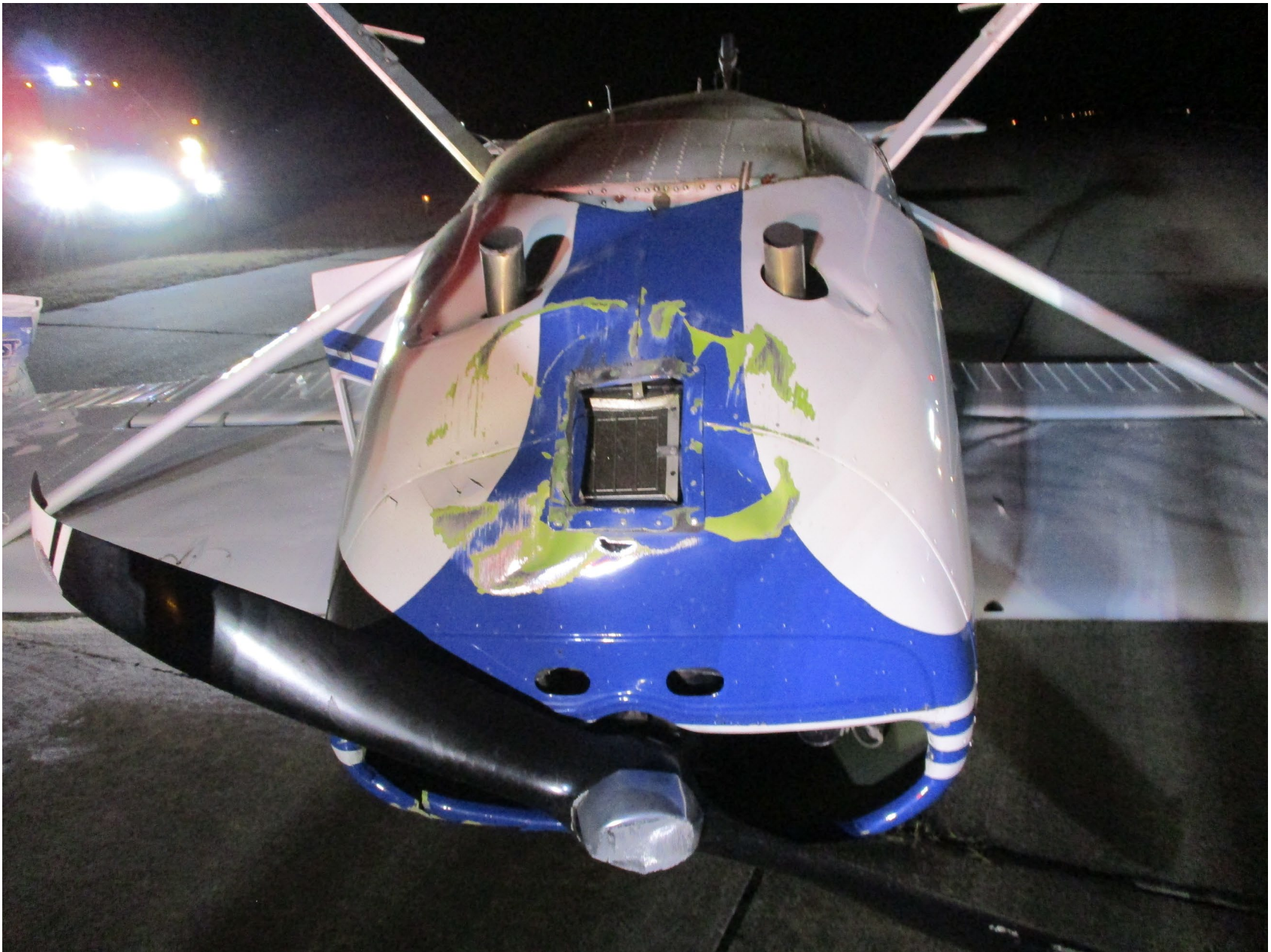
Photo 2 - Wrinkled Lower Cowling (Provided by FAA)
