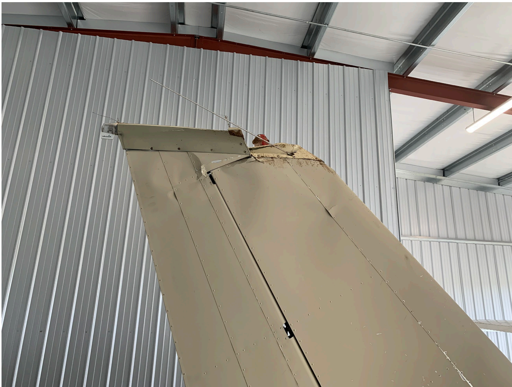
Photo 4: Accident Airplane / Damage to the vertical stabilizer – (Photo provided by the FAA)
