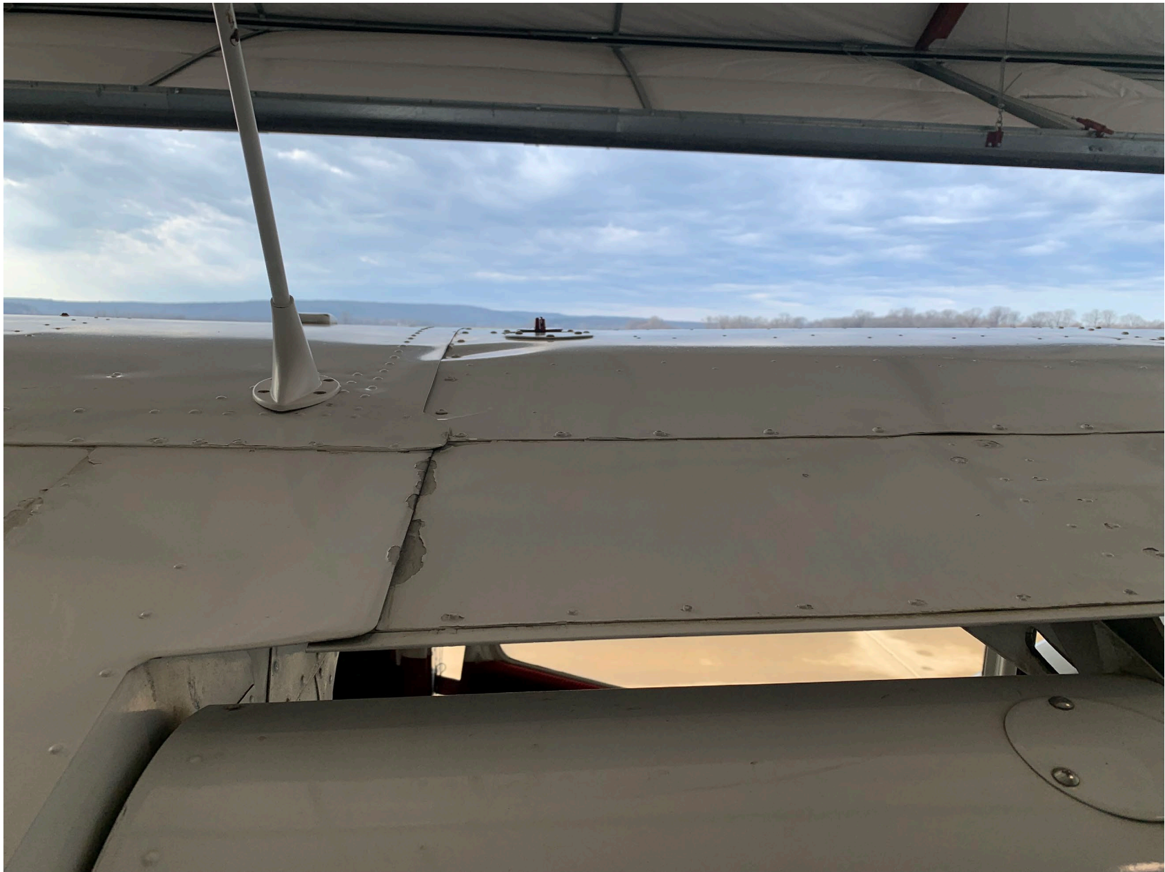
Photo 3: Accident Airplane / Damage to the top of the right wing – (Photo provided by FAA)
