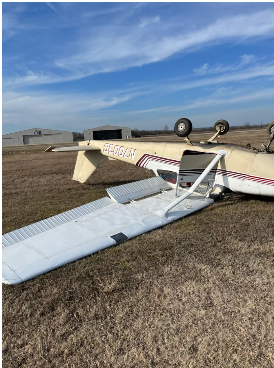
Photo 1: Accident Airplane / Damage to the left-wing strut – (Photo provided by FAA)
