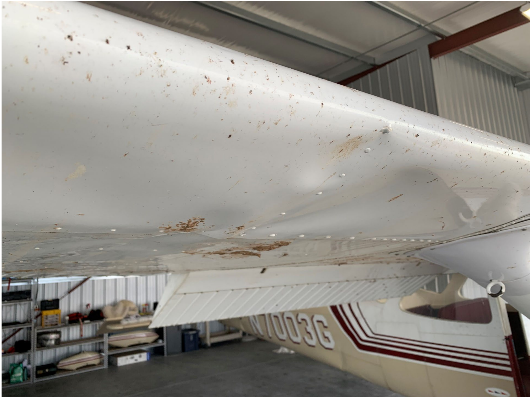
Photo 2: Accident Airplane / Damage to the right wing – (Photo provided by FAA)
