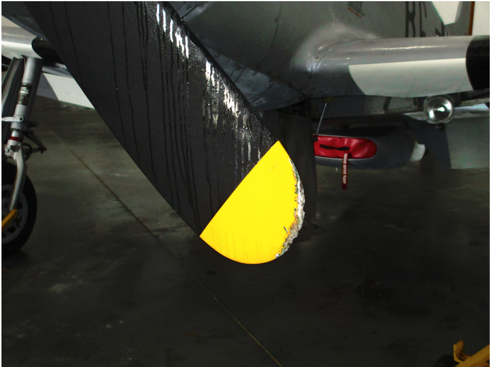
Photo 4 – N3333E propeller blade tip damage (Source: FAA)
