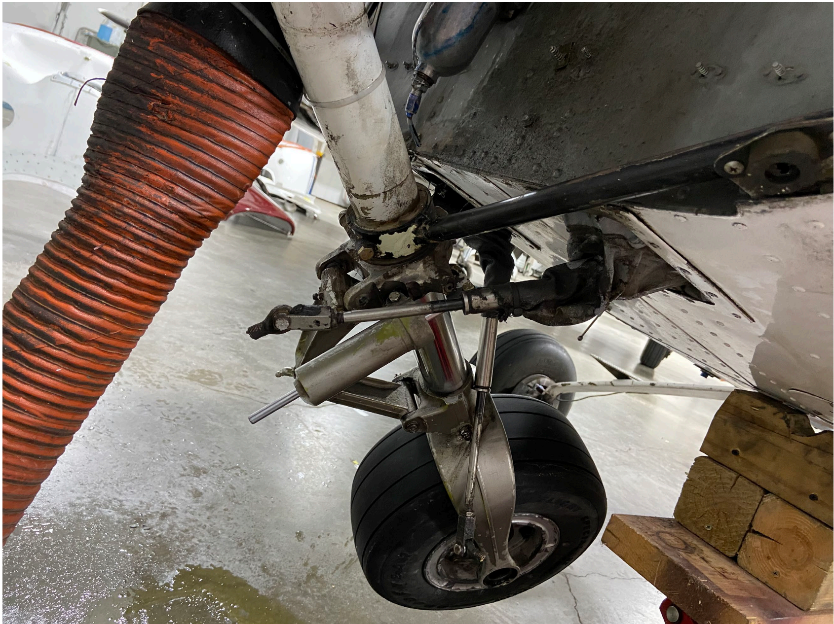
Photo 2 – Bent Nose Strut (Provided by FAA)
