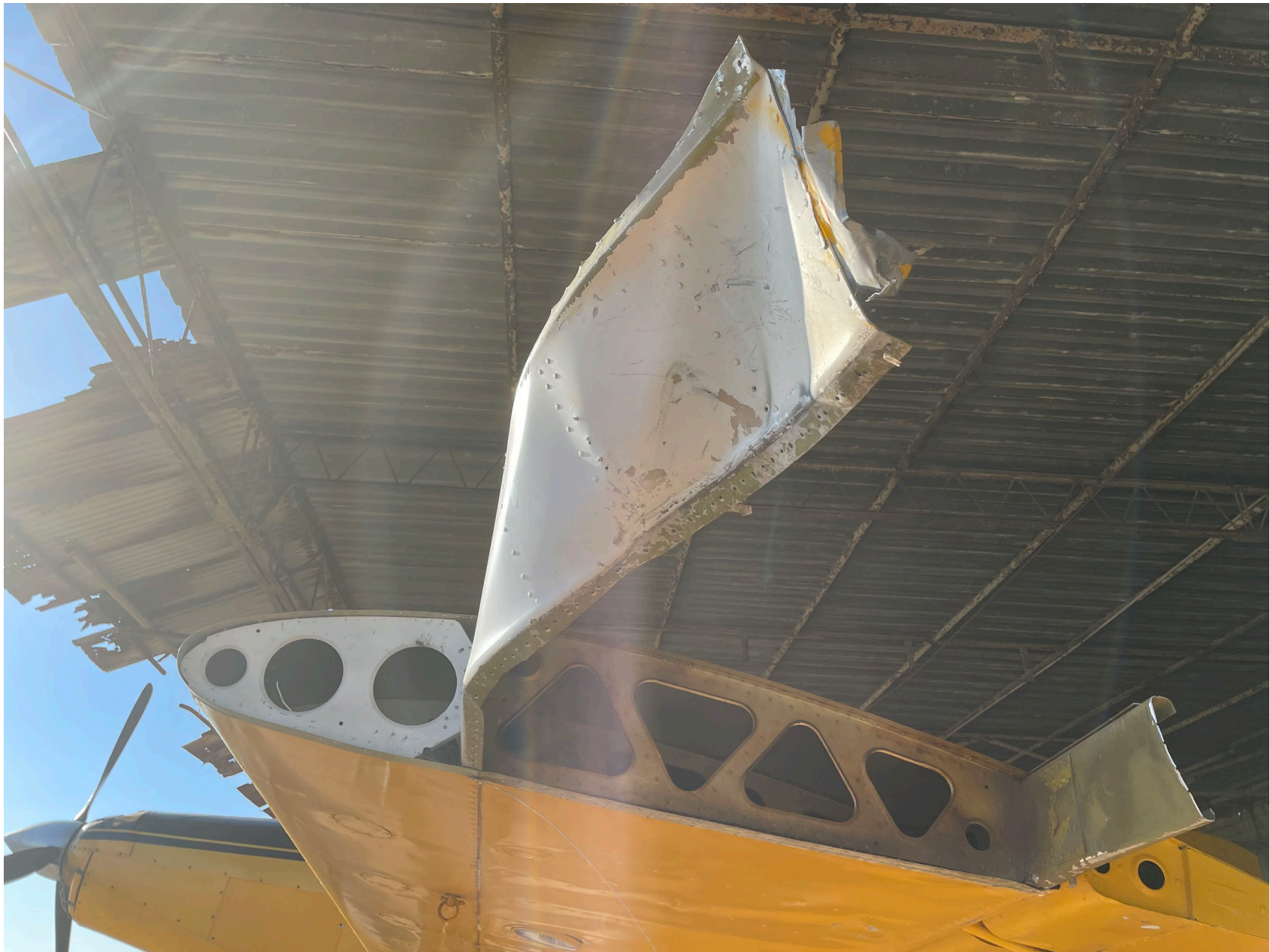
Photo 2: Accident Airplane / Close-up of left wing and main wing spar – (Photo provided by FAA)
