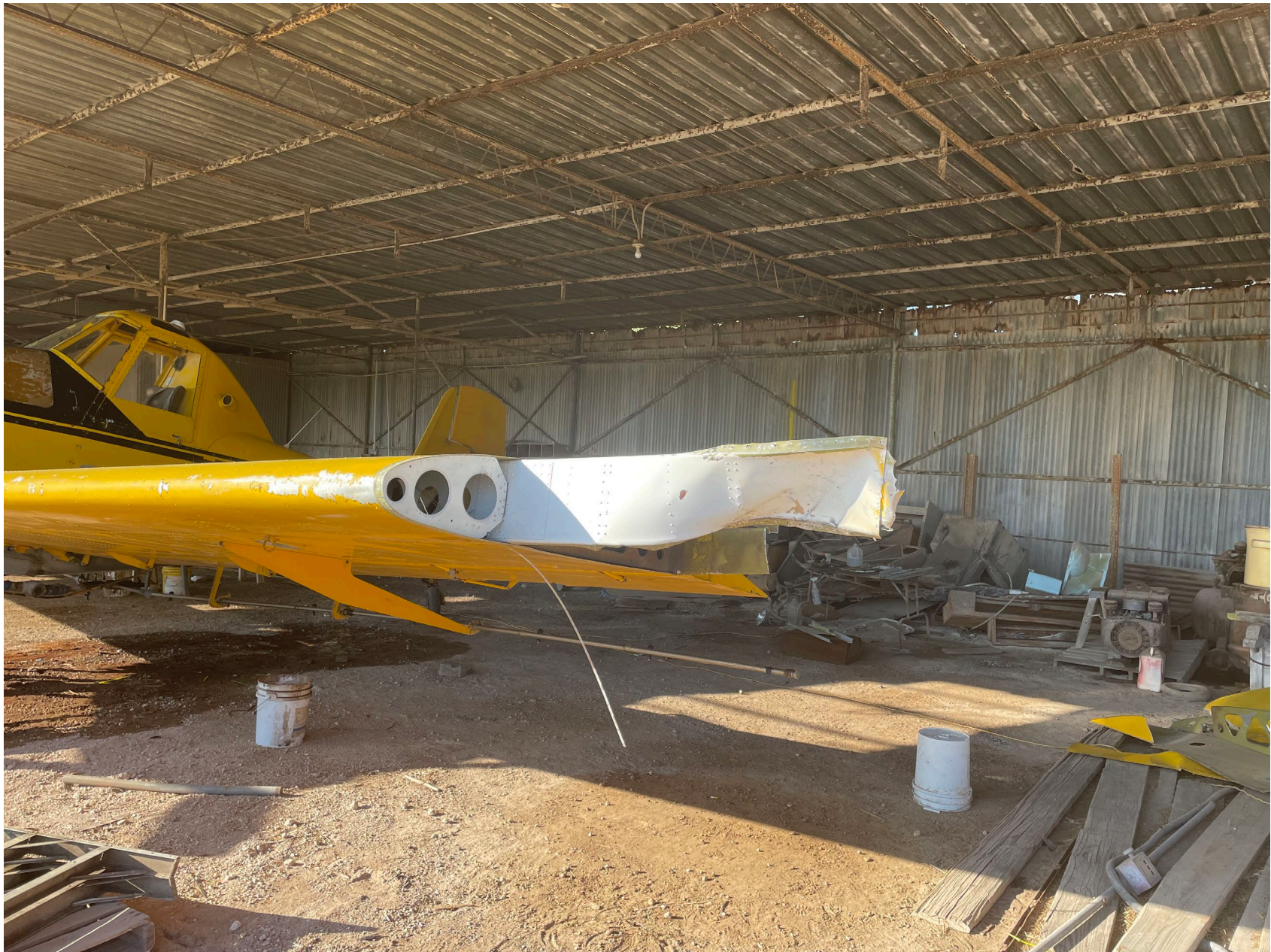
Photo 1: Accident Airplane / Left wing tip and main wing spar – (Photo provided by FAA)
