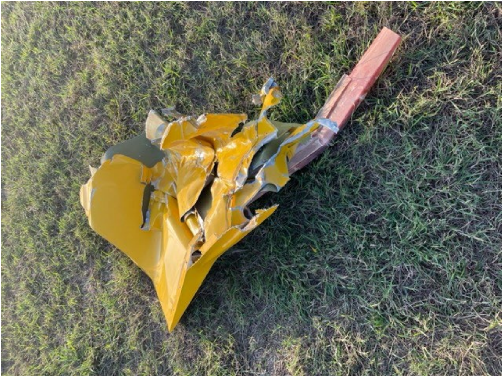
Photo 5: Damaged aileron - (Photo provided by FAA)
