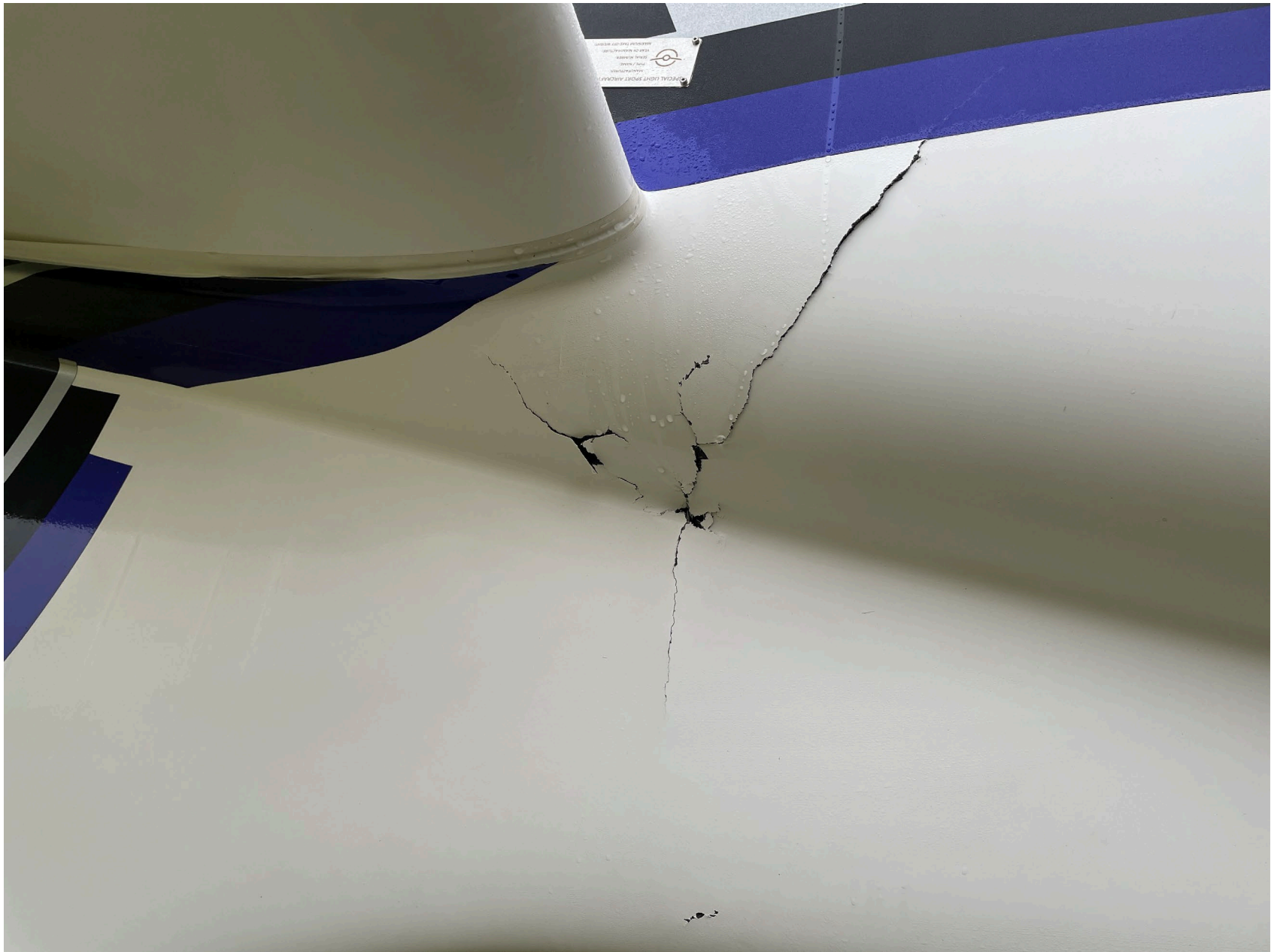
Photo 3 – Fractured empennage structure (Source: Federal Aviation Administration)
