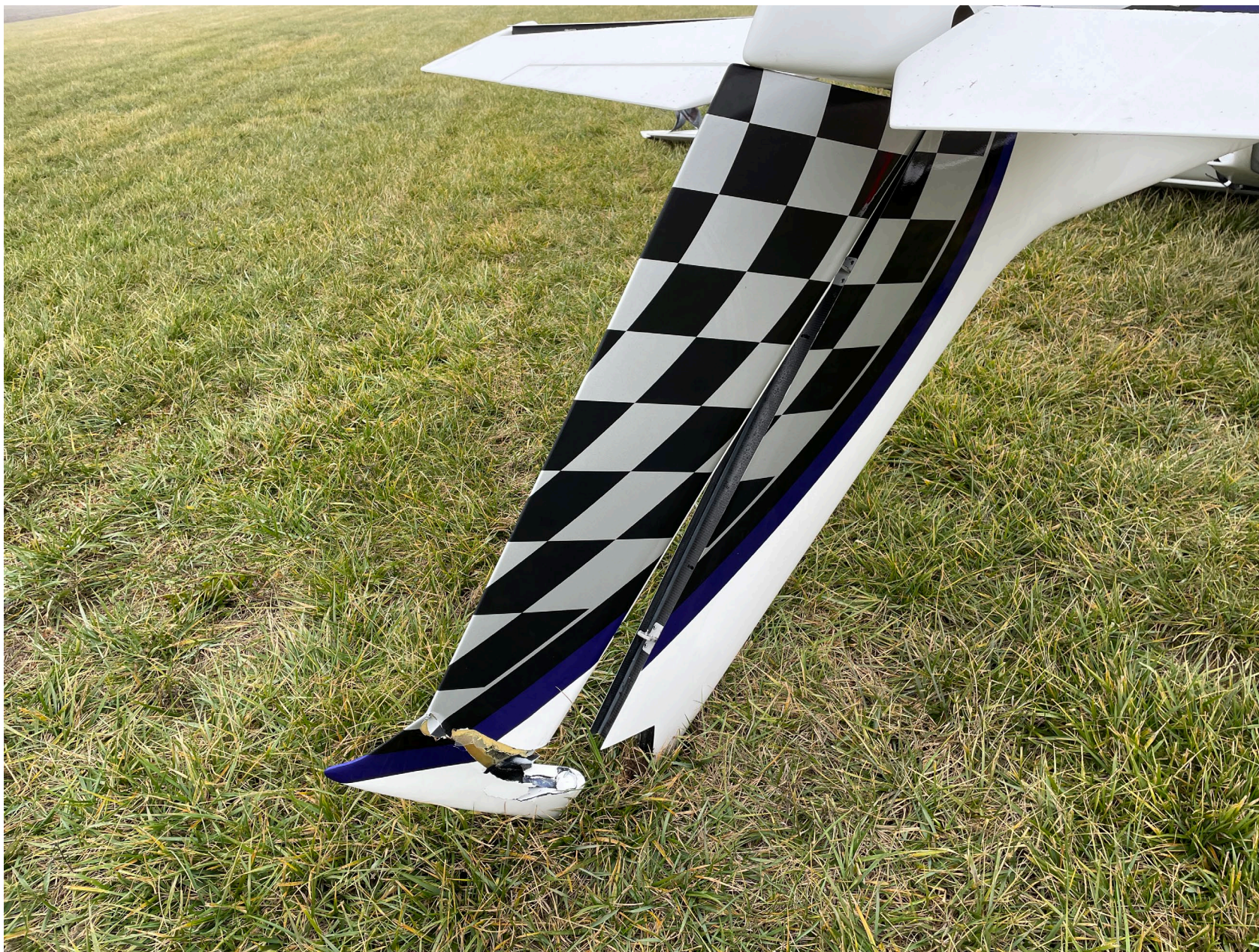
Photo 4 – Damaged rudder (Source: Federal Aviation Administration)
