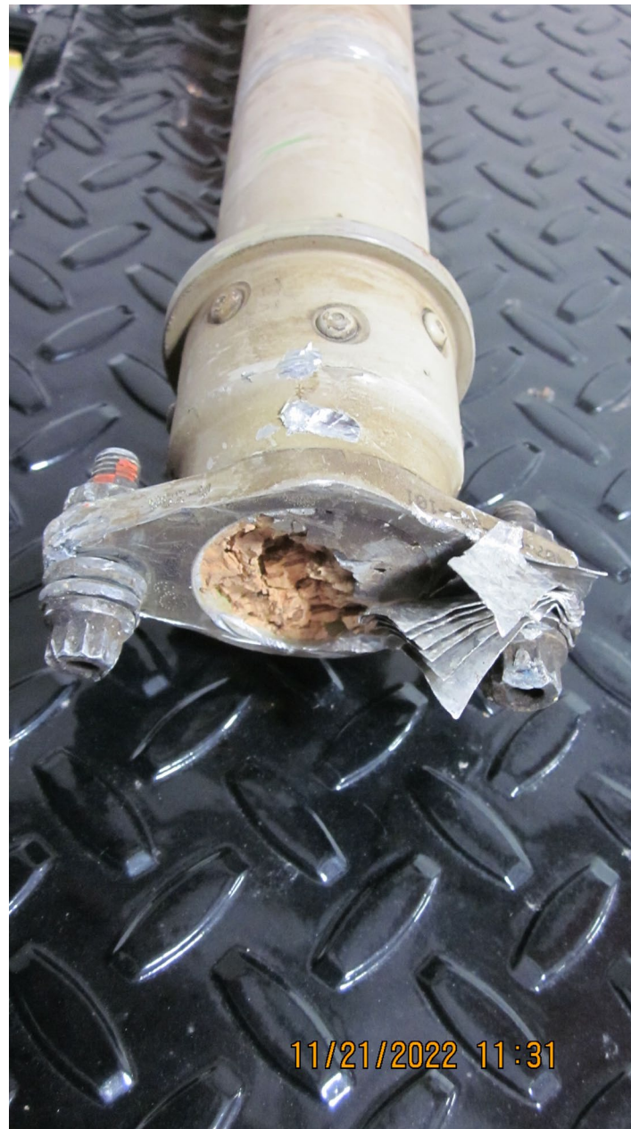
Photo 6 – Tail Rotor Driveshaft Coupling Damage (Photo Provided by Survival Flight)
