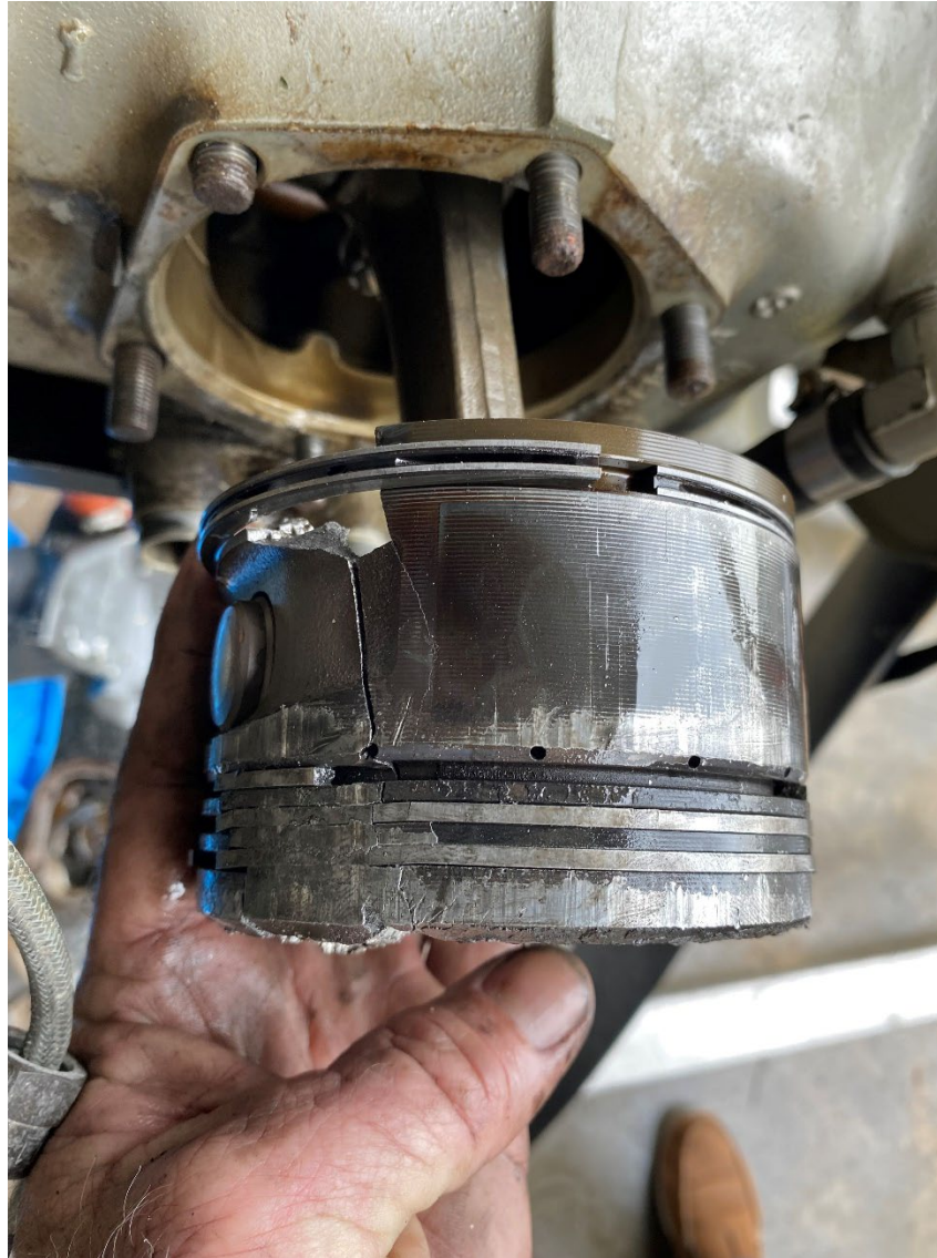
Photograph 5 - Number Three Cylinder Piston (Courtesy of Federal Aviation Administration)
